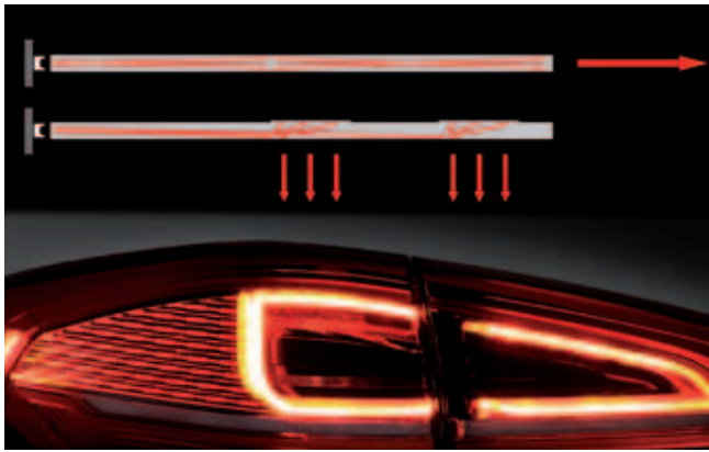
② Combination of the light curtain and EdgeLight systems
