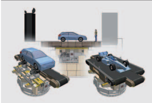
1 Interchangeable 3-/5-belt system for the 1:1 aeroacoustics vehicle wind tunnel
