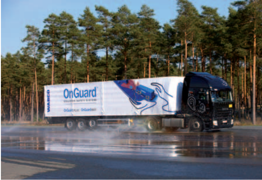
2 Test drive with ABS at the Wabco test track in Jeverzen (Germany)
