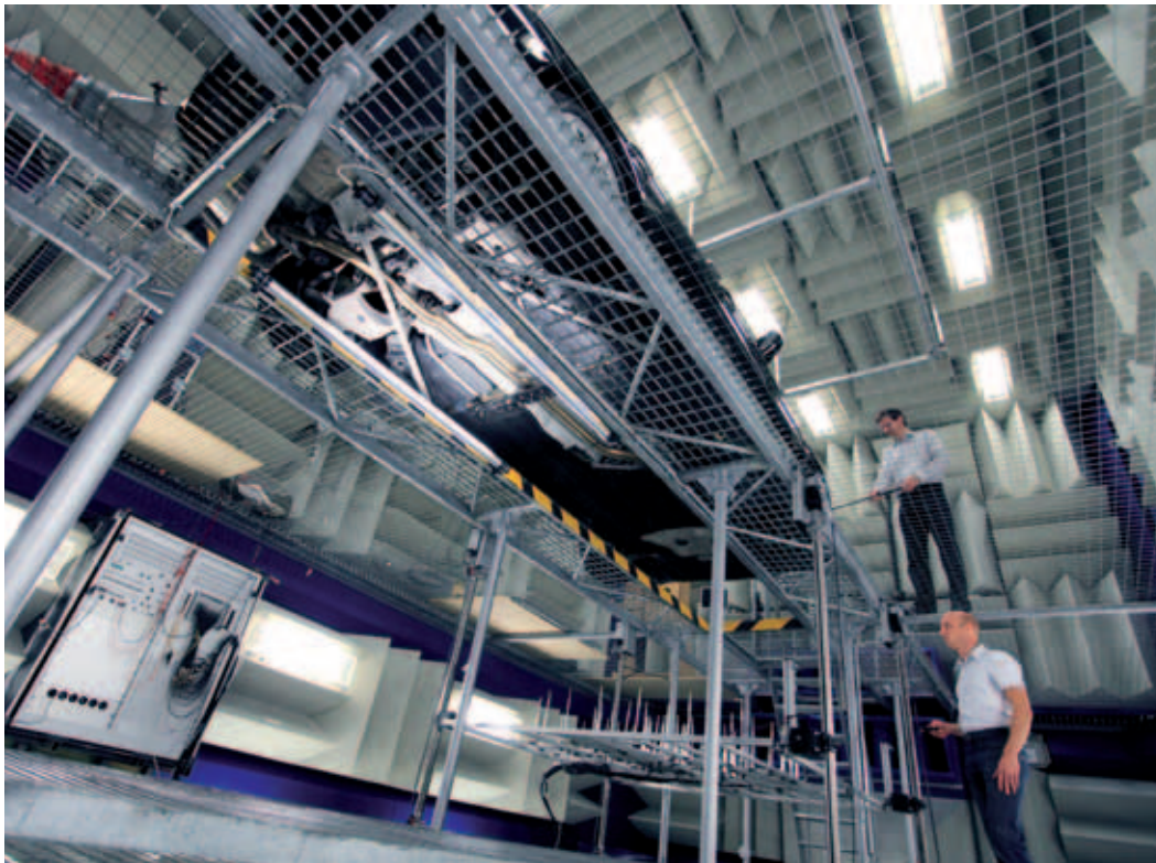
① Acoustic analysis of the car's underbody, using an underbody microphone array inside a full-anechoic room
