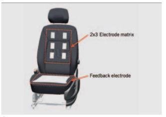
Capacitive electrodes integrated into the back of the driving seat, and a feedback electrode (driven ground) in the form of a seat cushion
