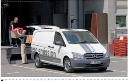
All-electric Mercedes-Benz Vito E-Cell with unchanged load compartment
