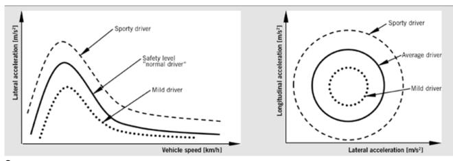
3 Reference samples regarding the correlation of vehicle speed and lateral acceleration and usage of Kamm's circle
