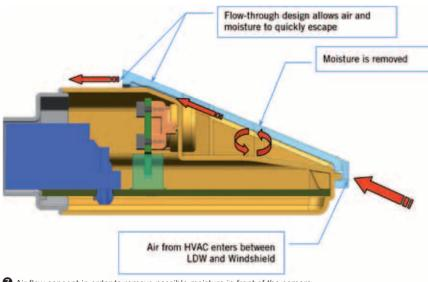
Air flow concept in order to remove possible moisture in front of the camera
