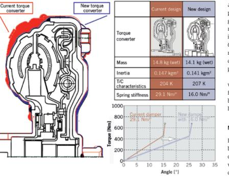
4 New torque converter with longer travel damper compared to the current design
