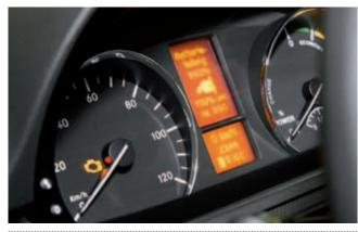
2 Power output display instead of the rpm counter
