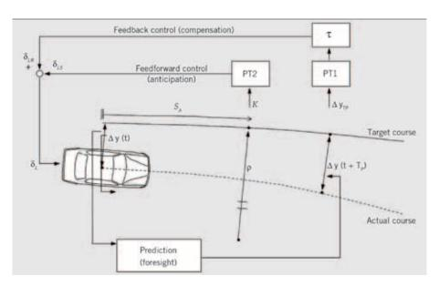
6 Control-theoretical driver model for vehicle lateral control
