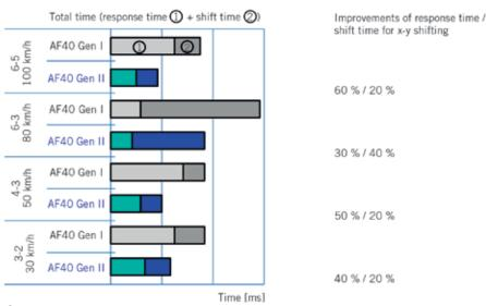
S Response time and shift time comparison for the current and the new transmission for four x-y down shiftings
