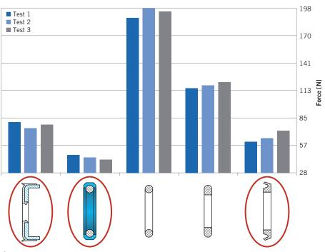
Basic tests with different transmission piston seals reveal big differences in their friction behavior – the solutions, which have so far delivered the best results, are marked in red (from left to right: composite transmission piston seal, a combination of O-ring with PTFE slip ring, O-ring, D-ring, as well as a U-packing; measurements of maximum friction at 500 mm/min, 5 bar sealing pressure and 23 °C)
