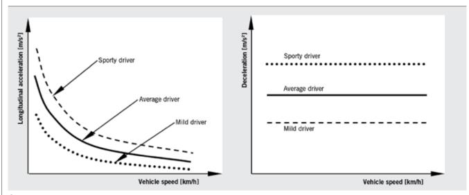
4 Reference samples regarding the correlation of longitudinal acceleration and deceleration to the vehicle speed
