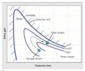
8 Conditions for stability in the coefficient diagram
