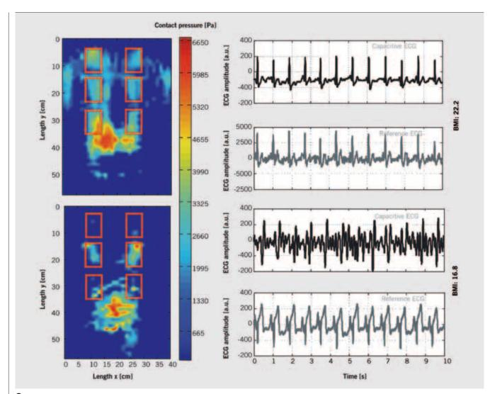
Ocntact pressures and related ECG signals for different body mass indices in artificial units [a.u.] (top: BMI in normal range, bottom: BMI below the normal range)
