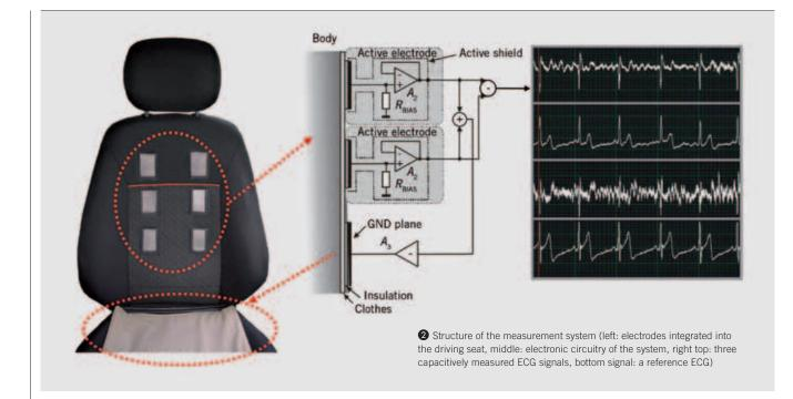
mode voltages on the body surface are not transmitted to the output of the system.
