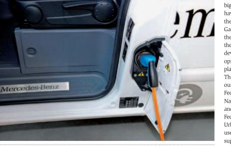
An immobilizer prevents the driver from setting the Vito E-Cell in motion during charging
