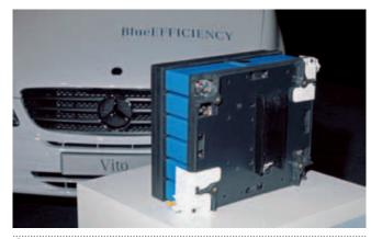
3 Lithium-ion batteries with an energy capacity of 36 kWh
