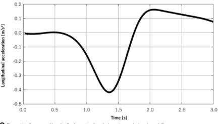
Obaracteristic curve of longitudinal acceleration during a transmission downshift
