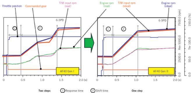
Time diagram for shift comfort improvement by eliminating the two-step response behavior with the new transmission
