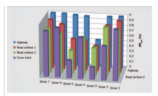
• QRS detection rate in the physiological range for different drivers and different test tracks; extreme acceleration and curved way of driving for Driver 3
