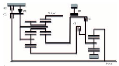
2 Power flow of the transmission with two brakes (B) and three clutches (C) as well as one one-way clutch (O)
