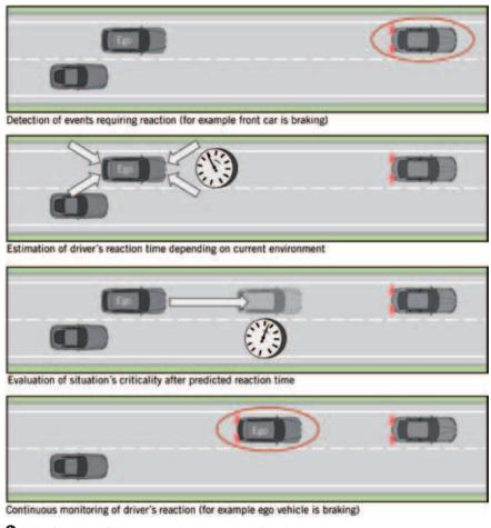
**1** Mode of operation of the emergency braking system in four phases
