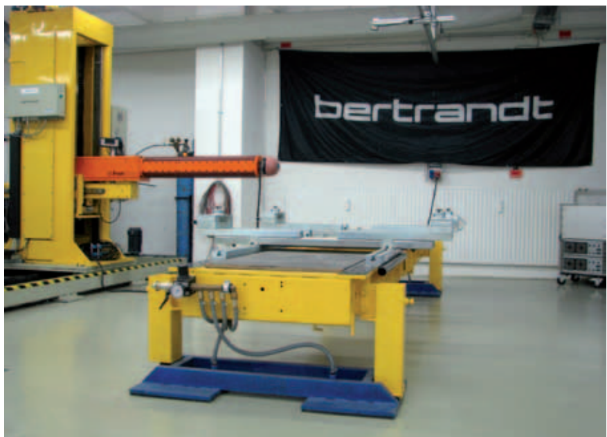
③ Test area for FMVSS 226 testing at Bertrandt in Munich
