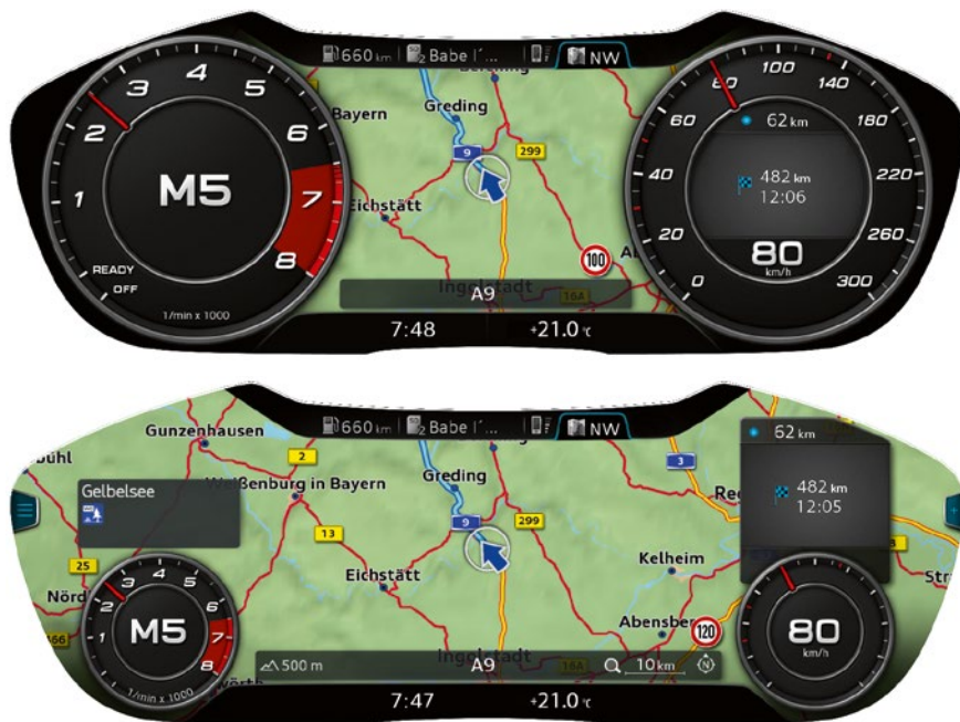
FIGURE 2 Classic display with large circular instrument dials (top) compared to the information view (bottom) focusing on the central section, here with the example of the navigation map (© Audi)
