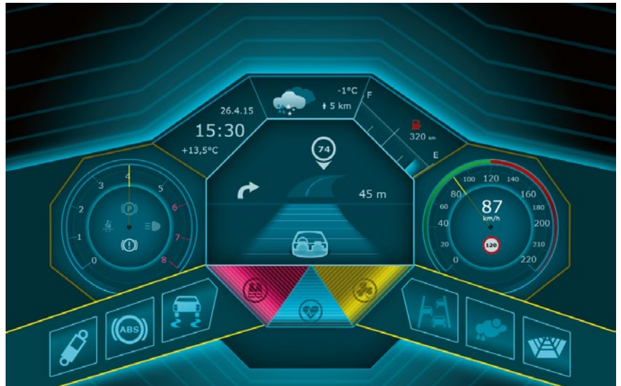
FIGURE 3 Example of the visualisation of the vehicle status on the instrument panel, including current weather data and future situations, such as bends and speed limits; a special feature is the representation of the recognised driving style in the colours magenta (safety awareness), blue (sportiness) and yellow (energy efficiency) (© Bertrandt)
