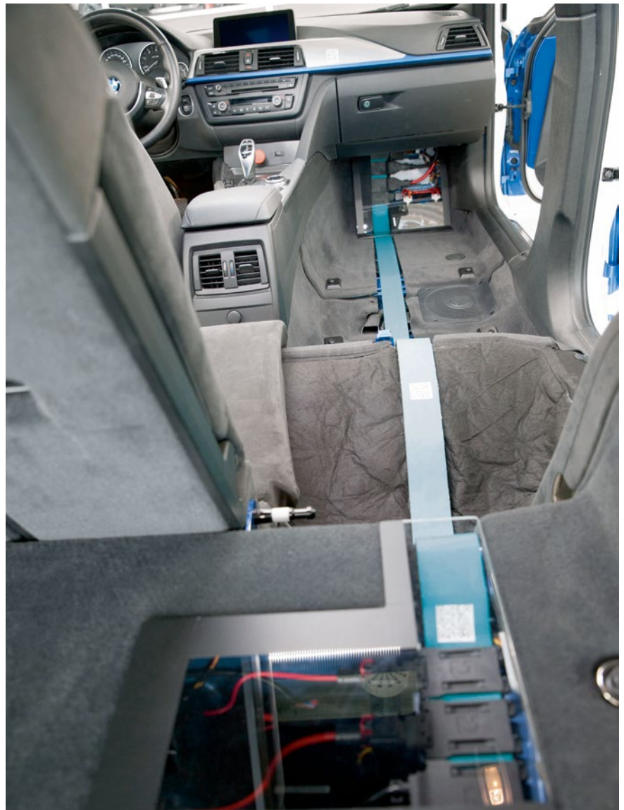
FIGURE 1 The triple-layer multi-bus in the Dräxlmaier smart KSK experimental vehicle includes front and rear connection technology (© Franz Haslinger | Dräxlmaier)
