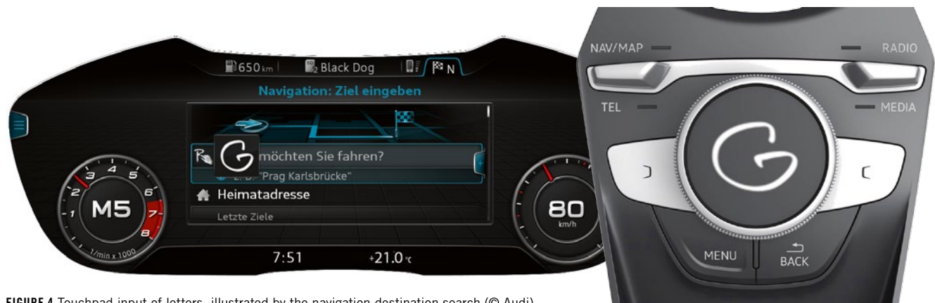
FIGURE 4 Touchpad input of letters, illustrated by the navigation destination search (© Audi)
