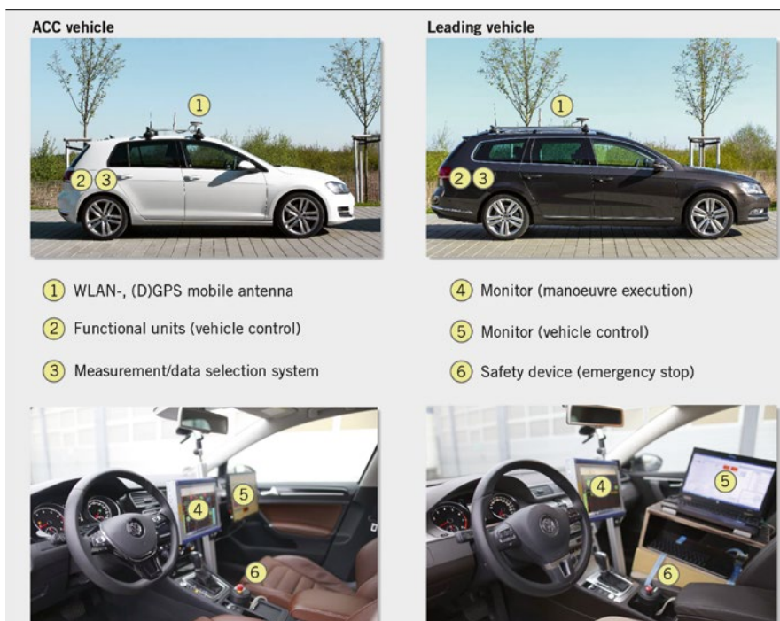
FIGURE 2 Test vehicles (ACC vehicle and leading vehicle) © Adrian Sonka, Christoph Nippold, Torben Pawellek, Louisa Liesner
