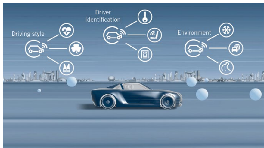
FIGURE 2 The three components of the adaptation of driver assistance system to the driver: driving style analysis – driver identification – environment recognition and evaluation (© Bertrandt)
