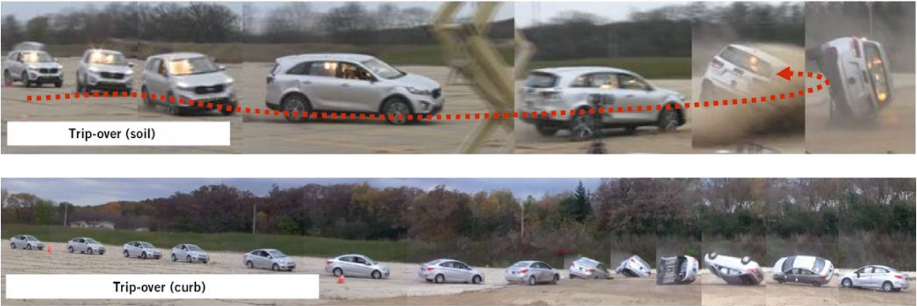
FIGURE 4 Panoramic view of steer-induced rollover test (© Hyundai)
