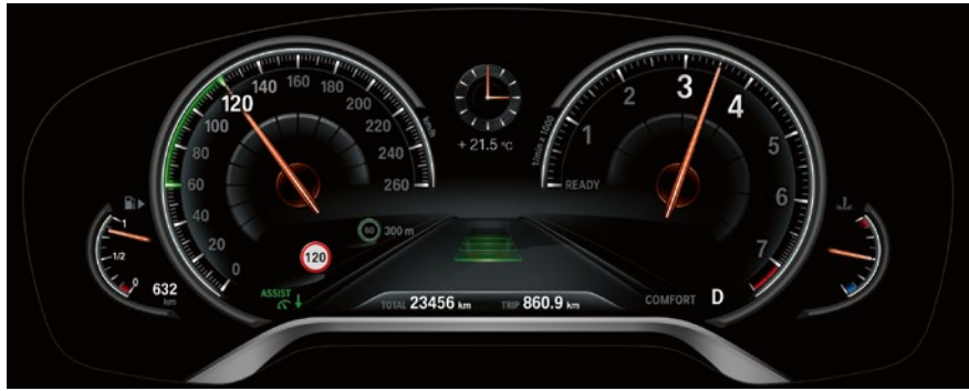
FIGURE 4 Upcoming speed limit for Speed Limit Assist framed in green (© BMW)
