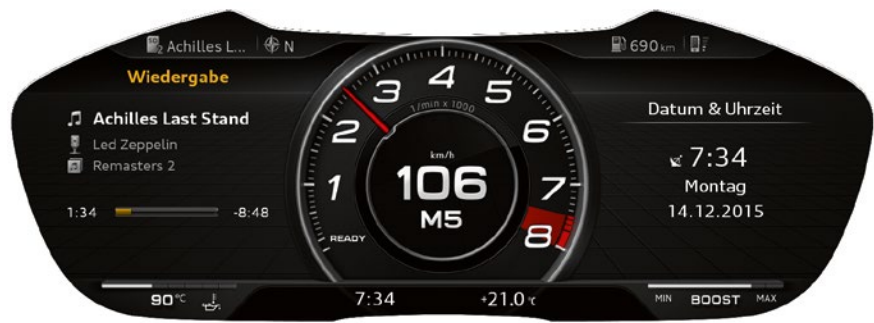
FIGURE 3 Audi TTS display with large revolution counter at centre (© Audi)
