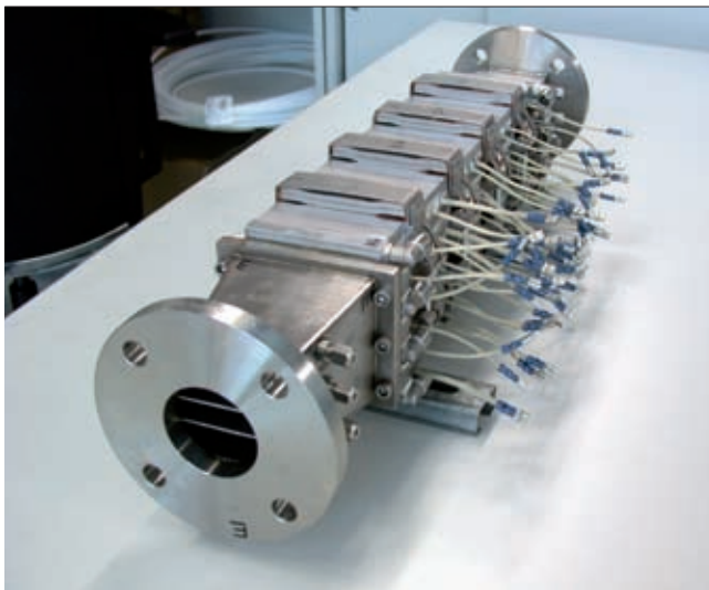
8 TEG functional model with flange-mounted test-bench diffusers
