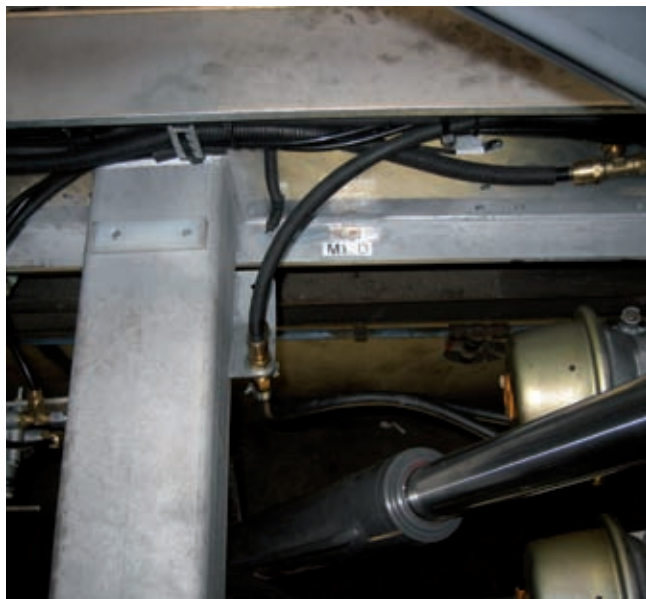
❶ Illustration of the measurement points M1_D and M5_D at the longitudinal beam of the trailer
