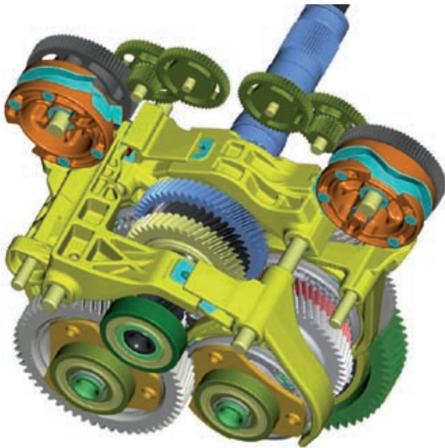
② Inner shift system with the parts intermediate gears, shift drums, linkages and shift forks
