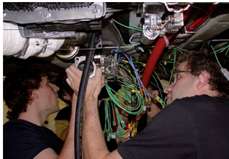
9 Vehicle integration of a TEG functional model
