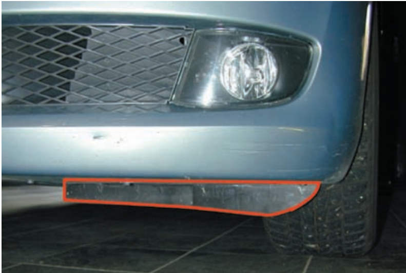
Figure 2: Bifid air dam of the model BMW E92 [3]
