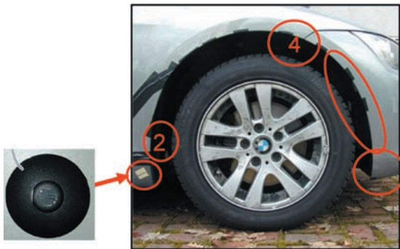
Figure 4: Surface microphone (left) and its positions on the vehicle (right, air dam not mounted), compare with Figure 8
