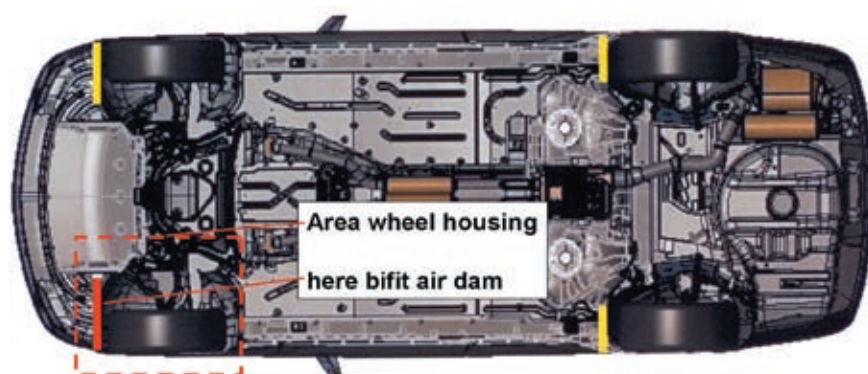
Figure 1: Vehicle undercarriage with the position of the air dam in front of the front wheel [2]
