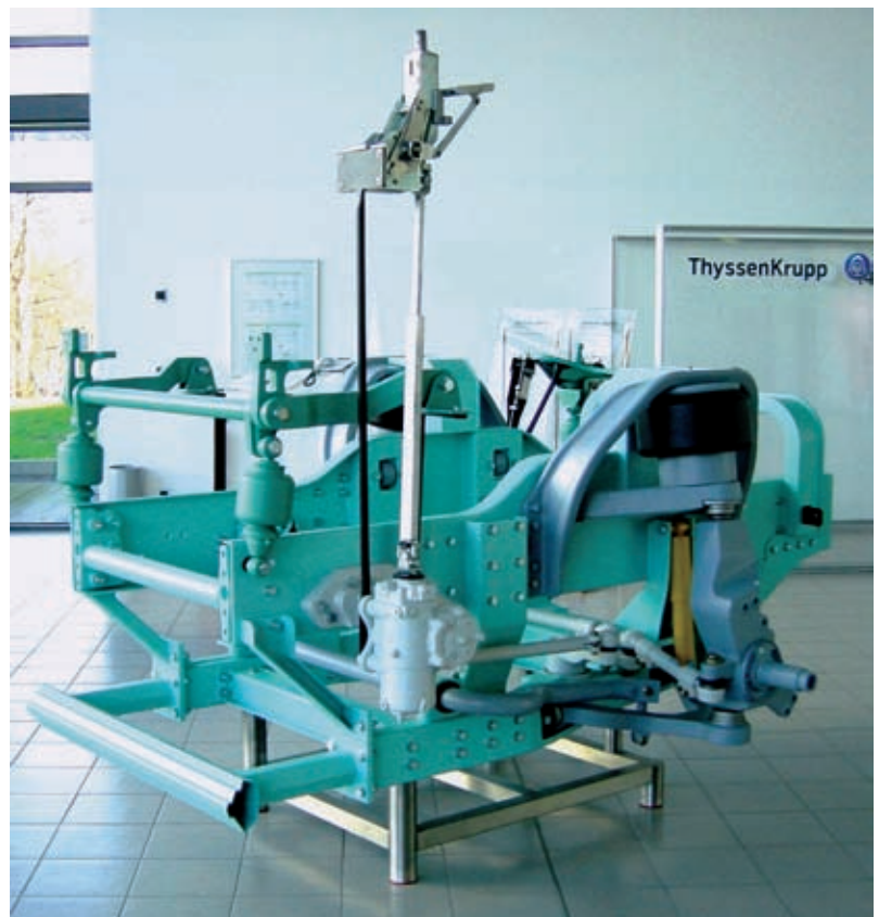
Figure 5: Truck show model of the structure featuring the independent wheel suspension
