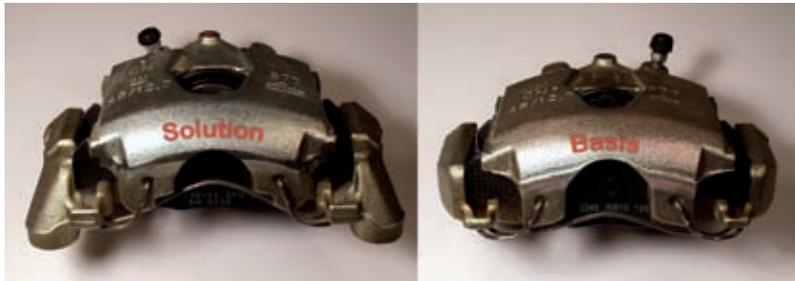
**Figure 10:** Structural imbalance due to additional mass on the brake caliper (solution, left, and basis, right)
