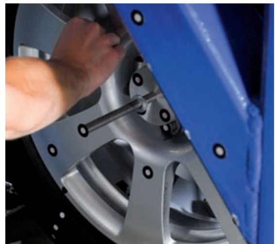
Figure 6: Preparing the axle for a six-dimension dynamic test on a chassis dynamometer rolling test stand
