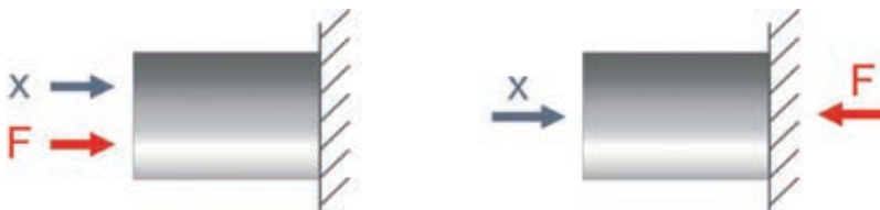
Figure 2: Input (left) and transfer (right) stiffness result from the nature of the experimental setup at the force F and the distance x
