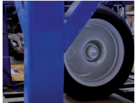
Figure 5: Assessment of an axle (with wheel) on a chassis dynamometer rolling test stand
