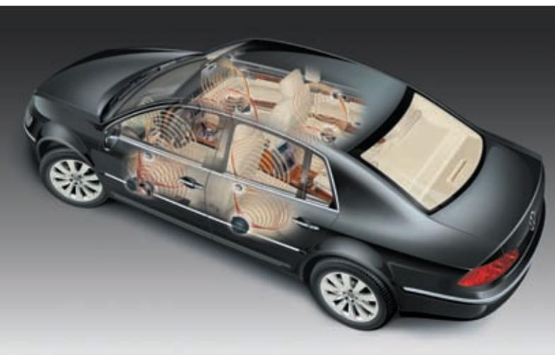
**Figure 4:** Dynaudio twelve-channel high-end sound system
