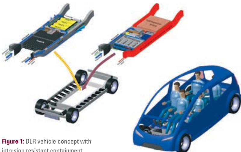
**Figure 1:** DLR vehicle concept with intrusion resistant containment
