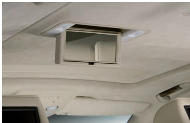
**Figure 5:** Retractable vanity mirrors for the rear-seat passengers
