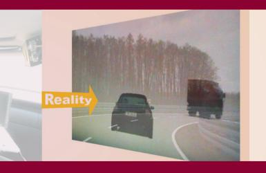
With the development of the Vehicle in the Loop, a test and simulation environment for driver assistance systems is presented by Audi, combining the advantages of a real test vehicle with the safety and reproducibility of driving simulators. Virtual outside traffic, road demarcations, or other simulated objects are visualized to the driver realistically.
