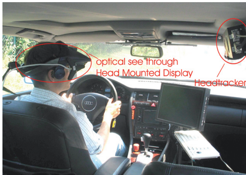
Figure 6: Head Mounted Display for the driver and head tracker in the test vehicle
