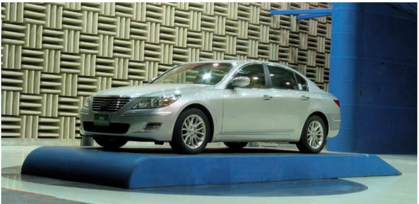
**Figure 1:** Genesis on a platform for underbody acoustic holography
