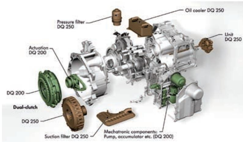
**Figure 1:** Design differences between six-speed transmission DQ250 with wet clutch and seven-speed transmission DQ200 with dry clutch
