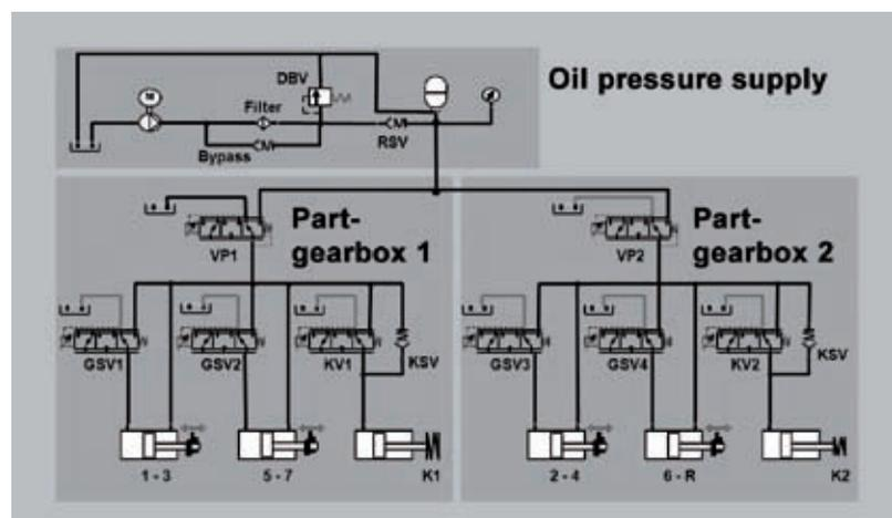
Figure 5: Hydraulics circuit diagram
