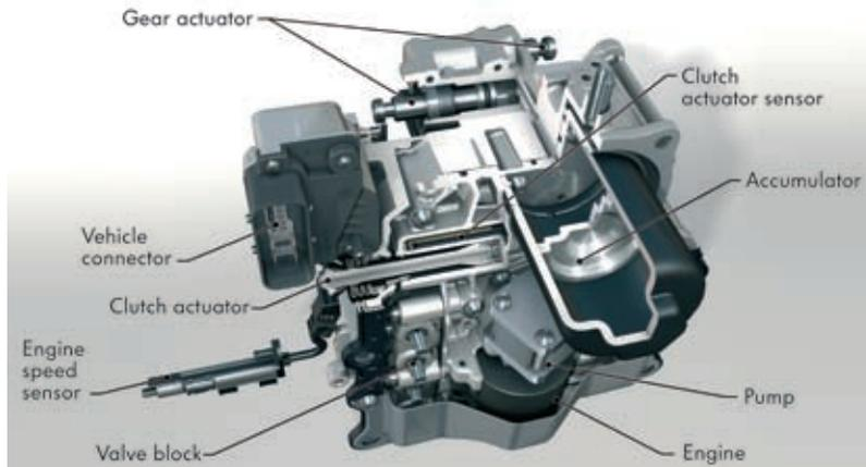
Figure 4: Mechatronics module
