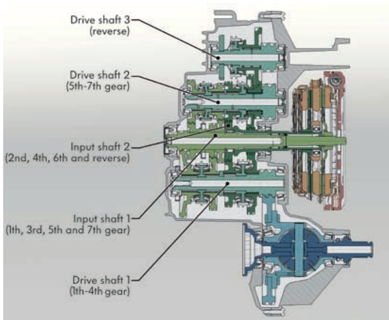
**Figure 2:** Schematic drawing of the seven-speed dual clutch transmission DQ200
