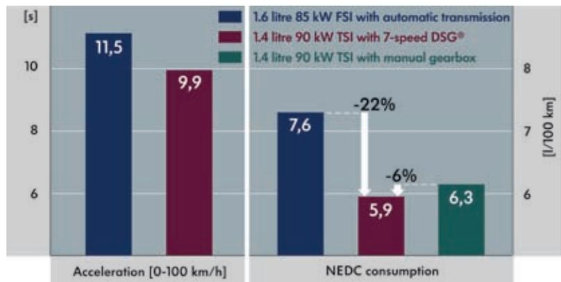
Figure 9: Comparison: VW Golf with petrol engine and automatic transmission
