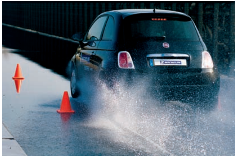
Figure 2: The tyre must be able to heat up immediately – for example during braking – in order to maximise grip
