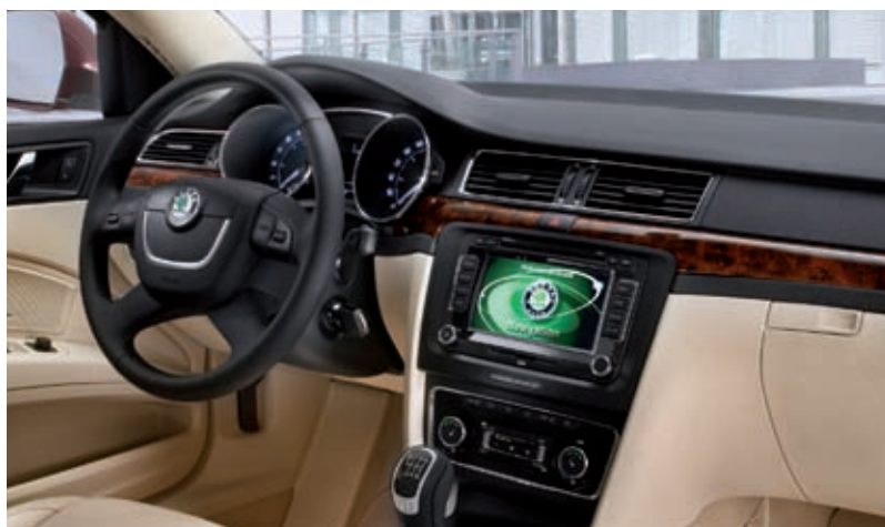
Figure 1: Part of the Superb's quality-feel is the fully foam-filled dashboard with its soft surface
