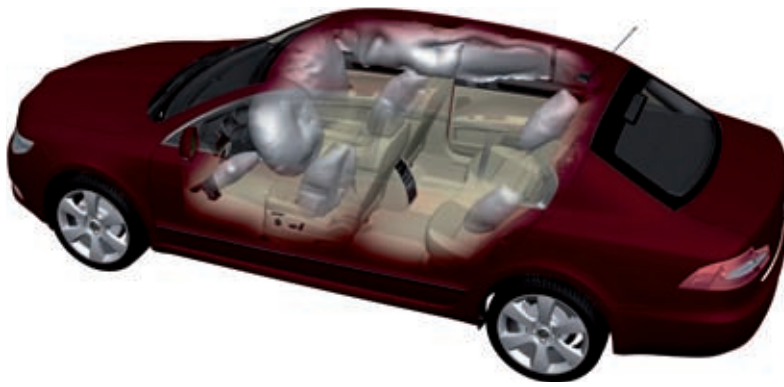
Figure 4: For the first time the Superb can be ordered with a driver knee airbag and rear side airbags
