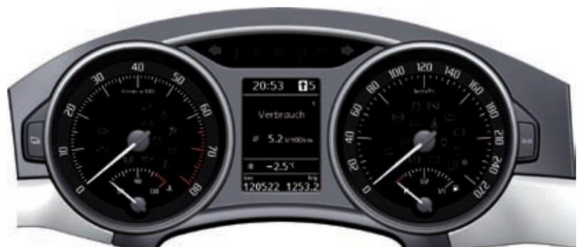
**Figure 10:** Indication of the used gear is shown in the cluster instrument as well as optimum time for gear change according to consumption
