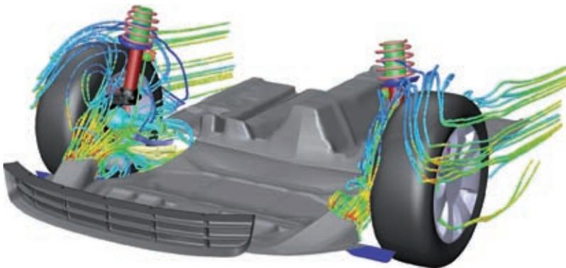
**Figure 3:** Simulation of the air flow to the brakes
