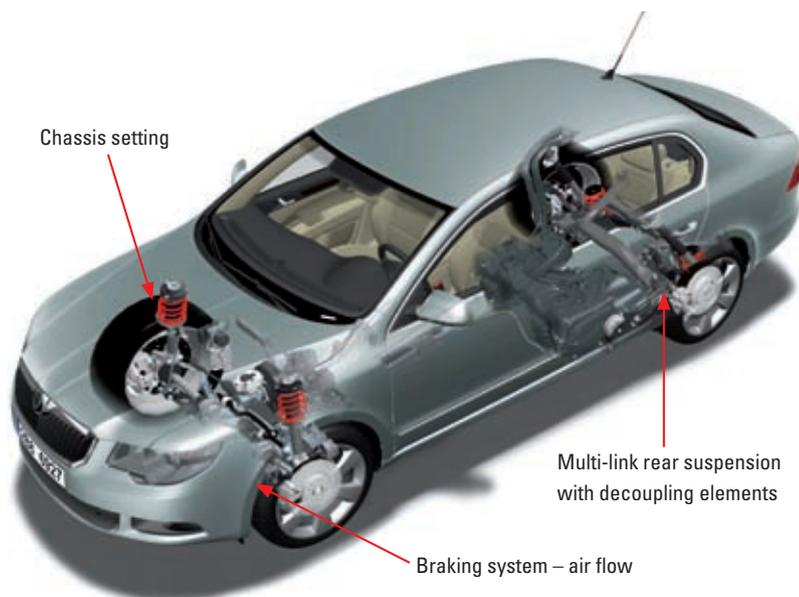
**Figure 1:** By carefully tuning the two axles with a special focus on interdependencies a highly compact and harmonic system with excellent driving properties was achieved
