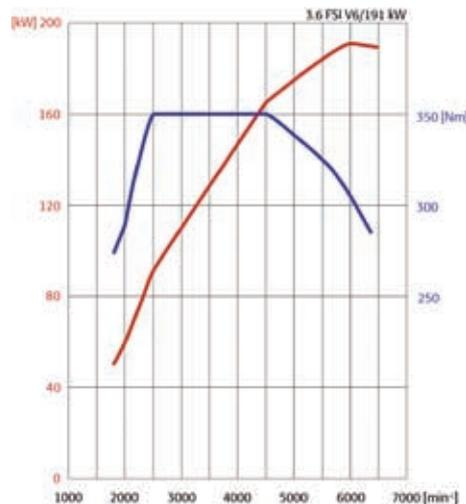
**Figure 5:** At 6000 revs/min the 3.6 liter V6 engine has a maximum power of 191 kW. The torque of 350 Nm is available from 2500 revs/min up to 4500 revs/min
