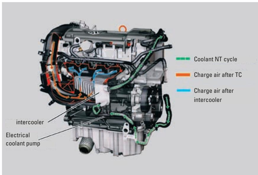
**Figure 4:** 1.4-l-TSI: Low-temperature coolant circuit at back of engine and air flow in charge air cooler
