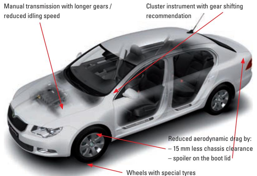
**Figure 9:** In the Greenline version the Superb has 0,6 l less fuel consumption per 100 km
