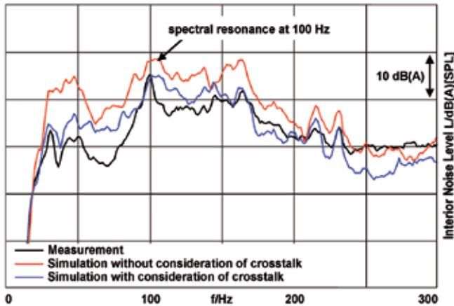
**Figure 4:** Comparison of measured and simulated interior noise with and without consideration of crosstalk
