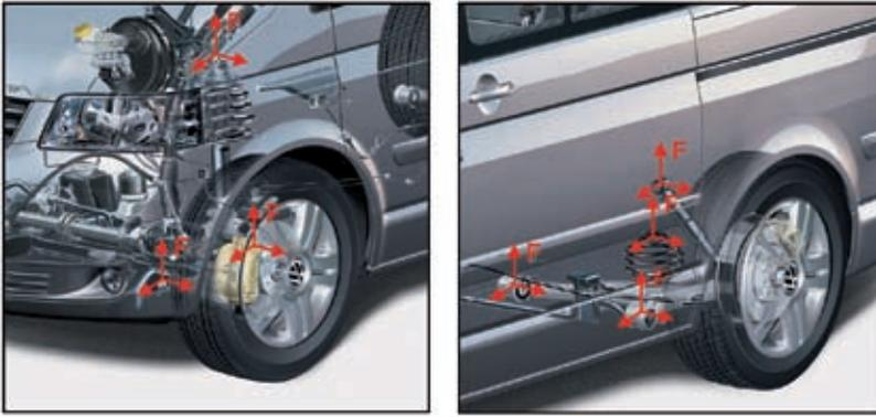
Figure 1: Force induction points at front and rear axle
