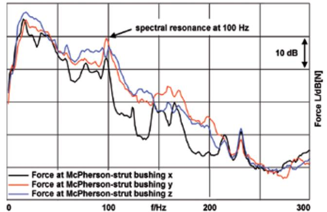
**Figure 5:** Calculated forces of the McPherson-strut showing a peak at 100 Hz
