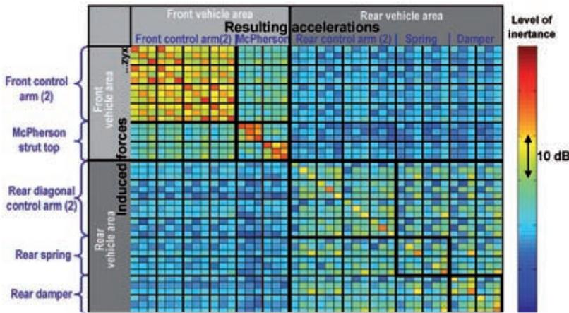
Figure 2: The inertia matrix describes the reaction (acceleration) of the vehicle body at the contact points on force induction at certain contact points. Colour shows average level of inertia function from 11 Hz to 355 Hz
