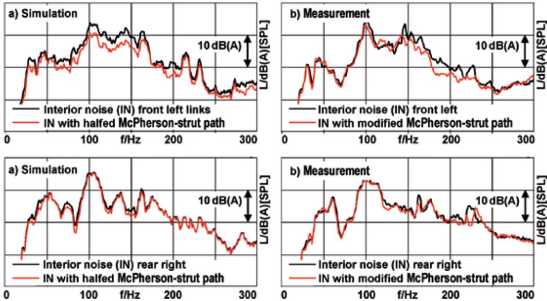
**Figure 6:** Effect of a modified noise path via the McPherson-strut on the measured and simulated interior noise
