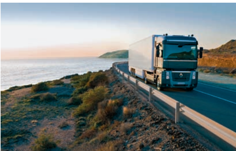
Figure 9: The model facelift measures on the Magnum are restricted exclusively to the cab. The powertrain with the two inline six-cylinder engines with just under 13 litres and 460 or 500 bhp and a manual 16-speed transmission and the option of an automated 12-speed transmission were taken over from the predecessor
