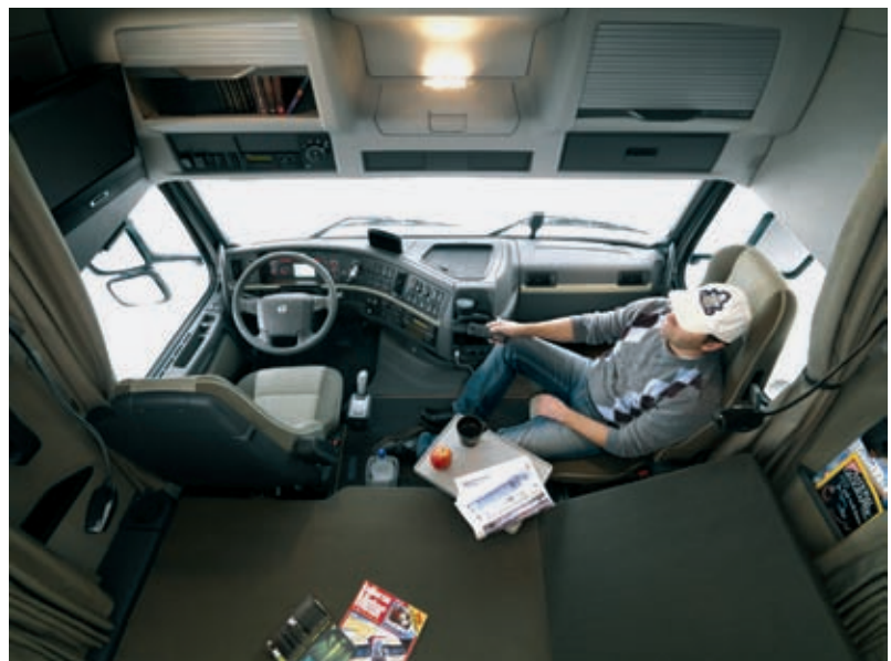
Figure 7: A newly designed frame above the windscreen provides more freedom of movement for the driver. An innovative feature is the reclining backrest of the lower bed. In addition, Volvo is providing the FH with more storage space and a variable interior lighting concept
