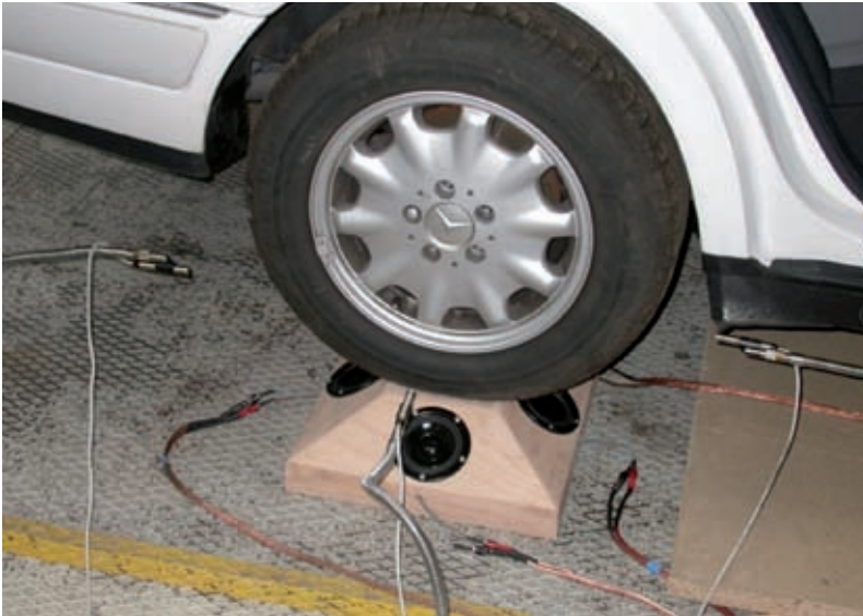
Figure 3: Speaker box and microphone array in a simulation of tyre-road noise on a test stand
