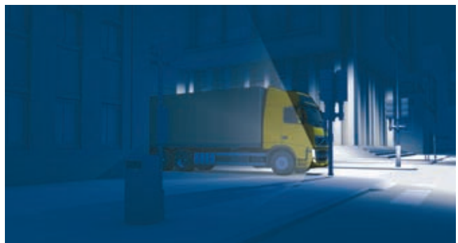
Figure 3: The new FH is the first truck to feature cornering lights. In the Volvo system, the cornering light is produced by a simple mirror installed at a 90° angle in the headlight. The light, which is activated as soon as the driver actuates the turn indicator, is conspicuous to warn pedestrians and cyclists that the truck may be about to turn
