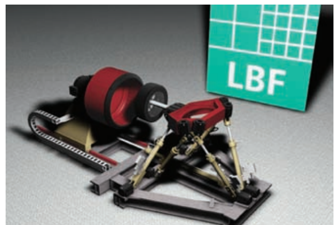
Figure 6: Overall view of LBF test machine for wheel accelerated life testing W/ALT
