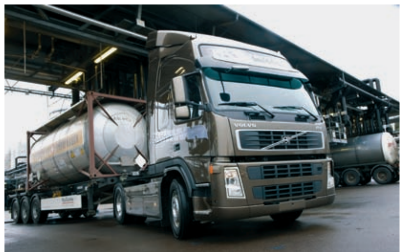
Figure 5: Volvo is equipping the heavy midsize class in future with a new 11-l inline six-cylinder engine with up to 430 bhp. Due to its increased load capacity, the FM is particularly interesting for weight-sensitive tank and silo transport. With the new Globetrotter cab, the new FM is also suitable for international use
