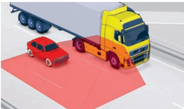
Figure 2: Volvo is the first truck manufacturer to introduce a Lane Changing Support system. An ultrasound broadband sensor monitors the traffic space directly to the right of the truck. If an obstacle is detected, the driver is warned by a visual signal in the A-pillar
