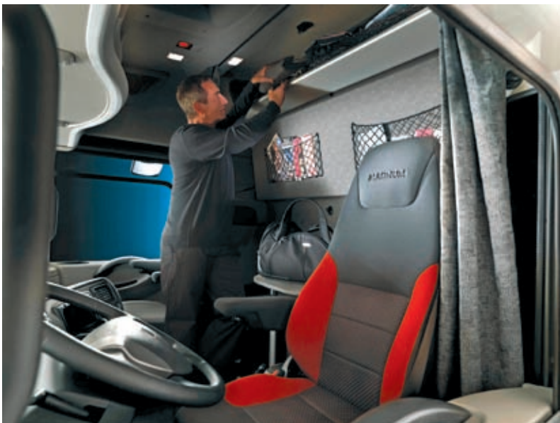
Figure 11: The working and living areas in the high-roof cab of the Magnum "New Generation" are separated both in their colours and in their equipment. Depending on the version, the Magnum has an adaptable seat/bunk arrangement that can be converted as required
