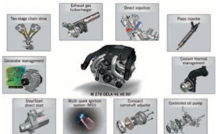
❶ Technologies used in the new M 278 V8 gasoline engine
