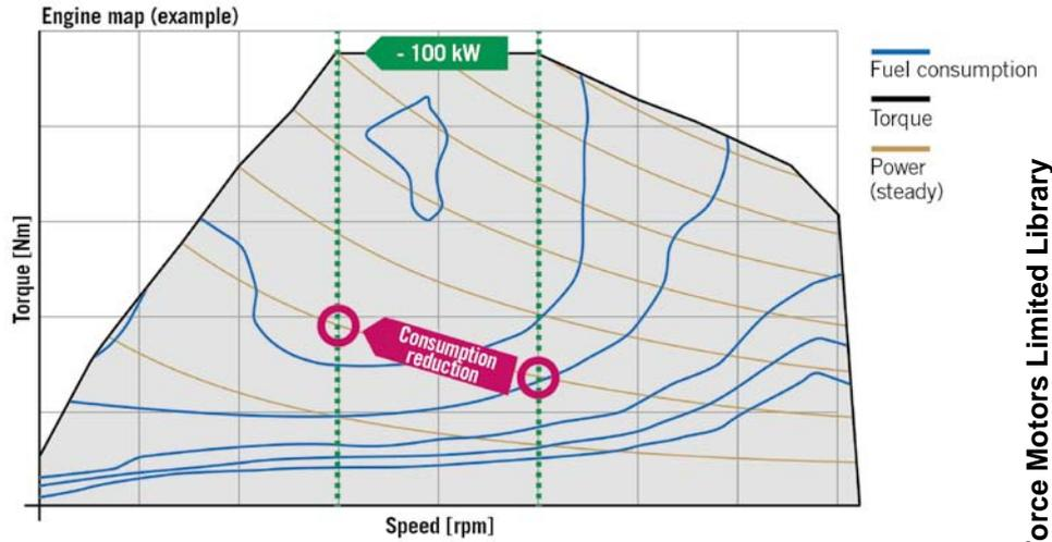
**FIGURE 1** If the engine speed is lowered by up to 400 rpm by means of very high-g geared axle ratios (green line), this leads to less performance and in particular torque reserves (black line) – even on very slight uphill gradients, the automatic transmission must downshift as a result in order to maintain the current driving speed (schematic view)
