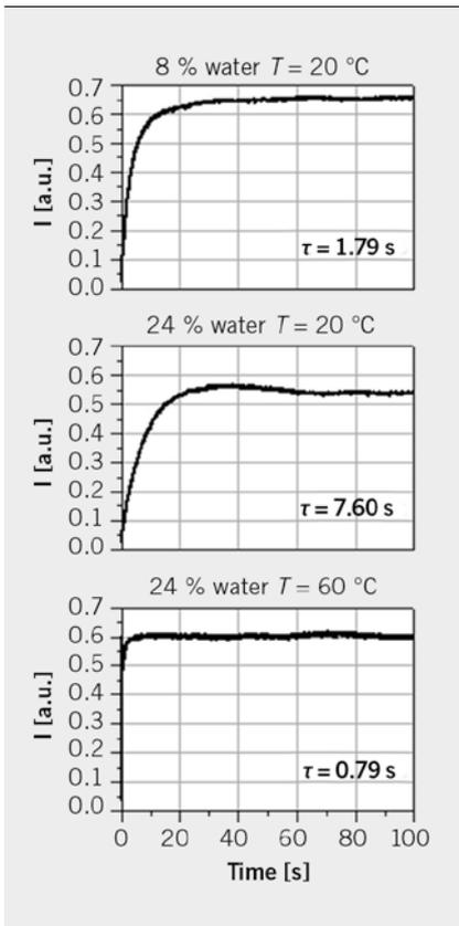
FIGURE 6 Stopped-flow measurement of mixture kinetics
