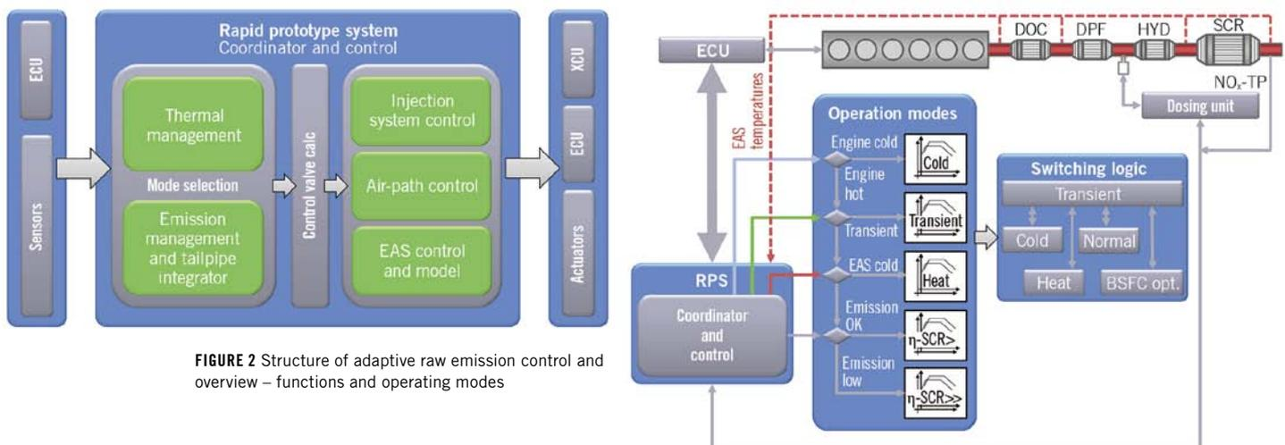
**FIGURE 2** Structure of adaptive raw emission control and overview – functions and operating modes
