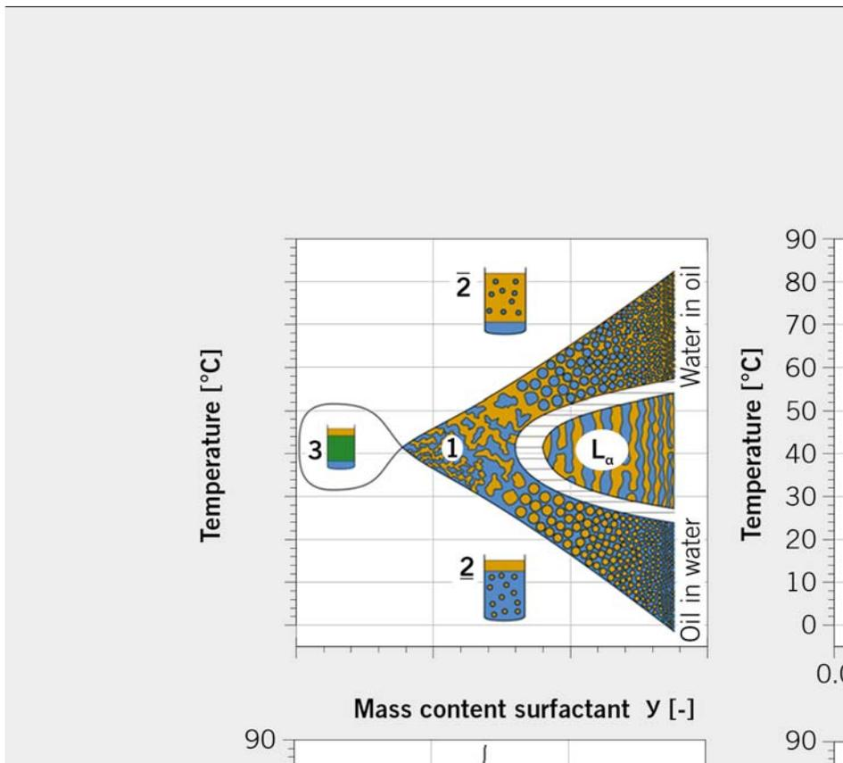
**FIGURE 2** Phase behaviour of micro emulsions (schematic (upper left): with 8 %, 16 % and 24 % water; composition of real systems: Water/Ethanol/Ammonianitrate – Diesel – Oleic acid/Monoethanolamin/ Wallamid OD4 with variable contents
