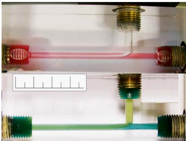
FIGURE 5 Diesel-water mixing behaviour without (top) and with (bottom) surfactant
