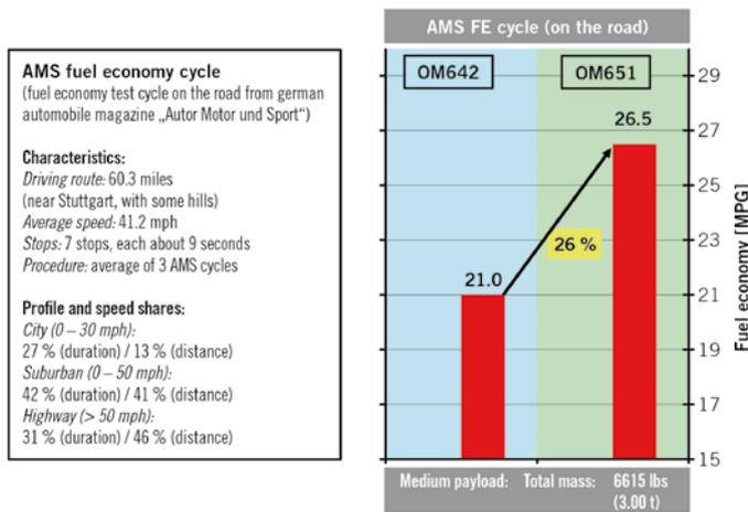
FIGURE 9 Fuel economy results at the AMS FE cycle (real test run on the road near Stuttgart, Germany)
