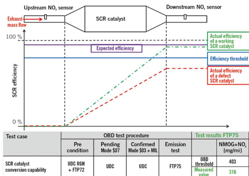
FIGURE 7 Diagnostic principle and related comparison of SCR efficiency and OBD test results of SCR catalyst efficiency diagnosis for GVWR > 10,000 lbs
