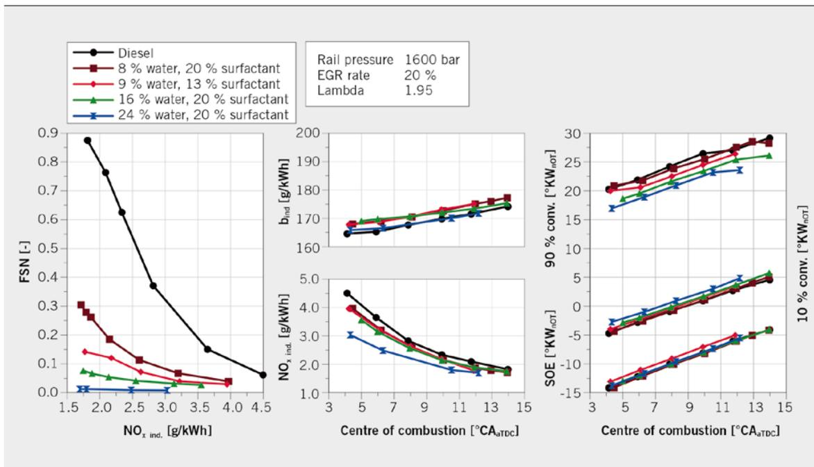
**FIGURE 3** Comparison of premixed micro emulsions at part load point B50
