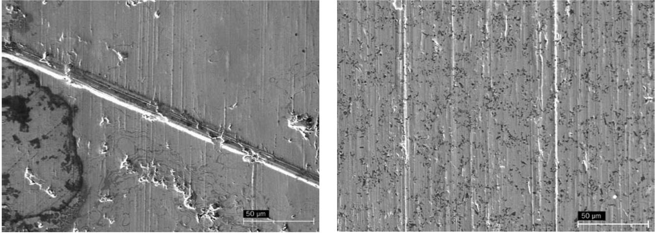
FIGURE 3 Comparison of an electroplated NiSi carbide coating and a Sprayfit liner after several motorcycle races: Sprayfit (left), Nikasil (right)
