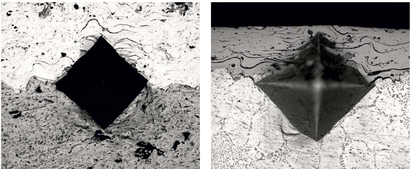
FIGURE 4 Result of adhesion test using an indenter: Sprayfit liner (left) versus arc-sprayed direct bore coating (right)
