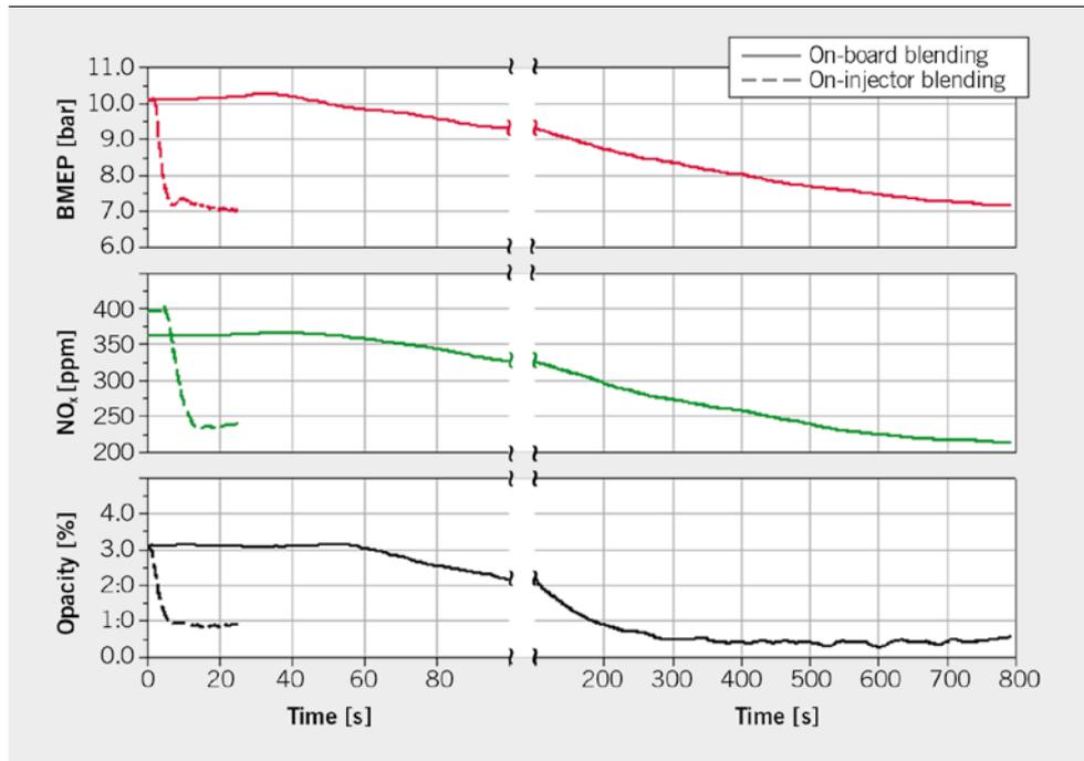
**FIGURE 8** Temporal change of pme,  $\text{NO}_x$  und opacity with water mixture activation
