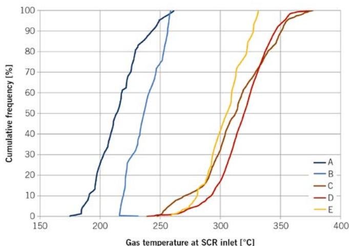
**FIGURE 3** Cumulative frequency of the gas temperature at SCR inlet for cycles A to E
