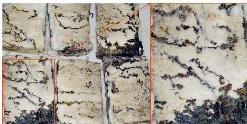
**FIGURE 4** Oil saturation behaviour and formation of oil discharge „channels“ in fleece fabric
