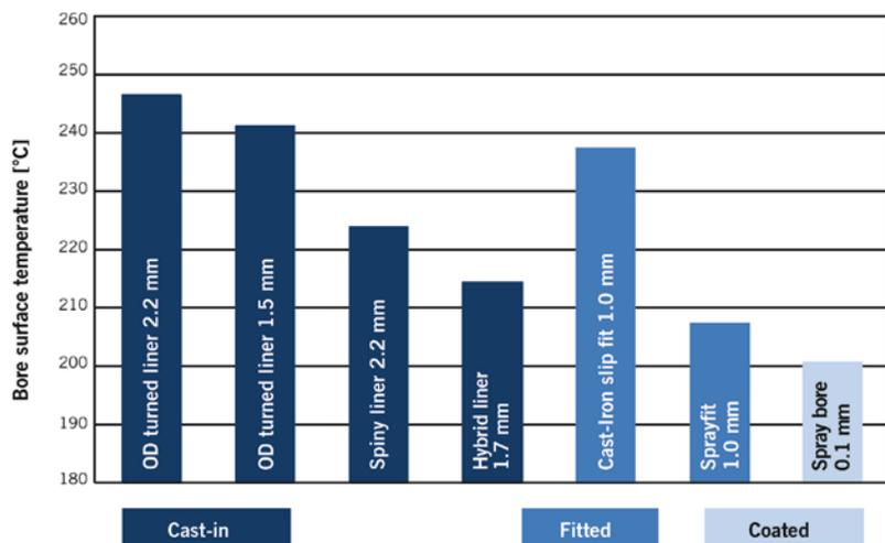
FIGURE 2 FEA model of the cylinder wall temperatures of different liner technologies
