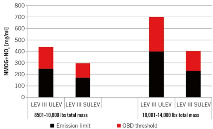
**FIGURE 6** Comparison LEV III ULEV and SULEV emission limit (MDV) and related OBD threshold limits (NMOG+NO<sub>x</sub>) for SCR catalyst diagnosis
