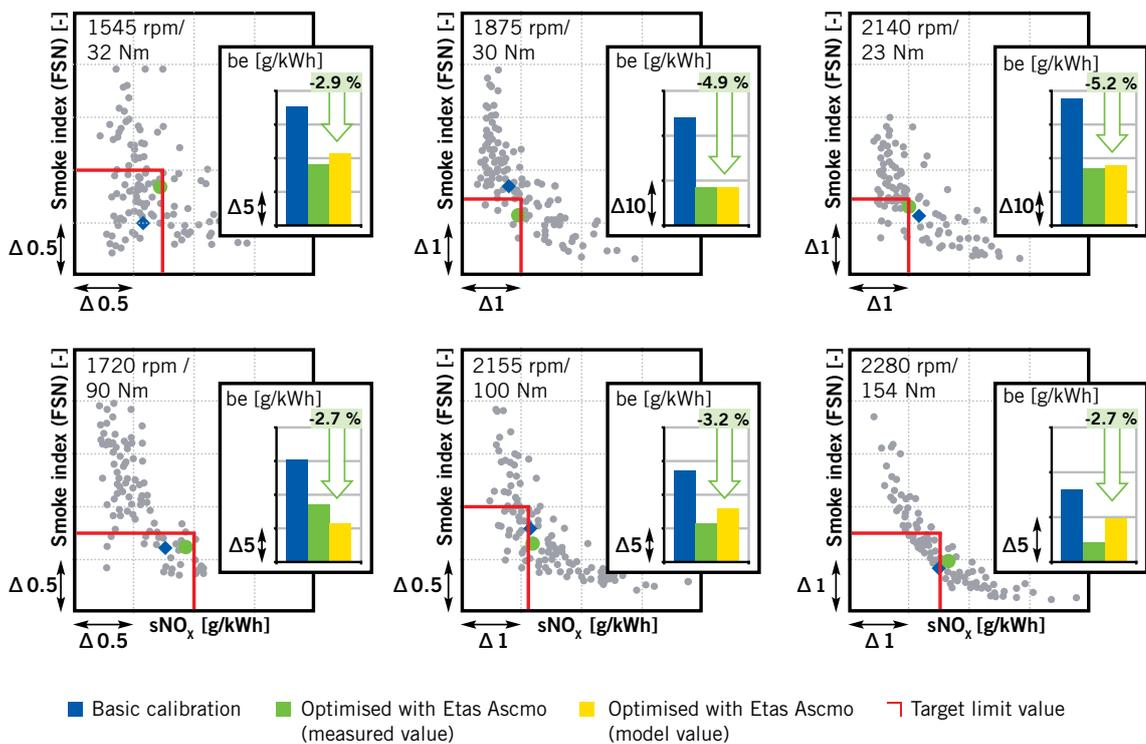
FIGURE 4 Optimisation results based on measurements taken at six operating points on the engine test bench
