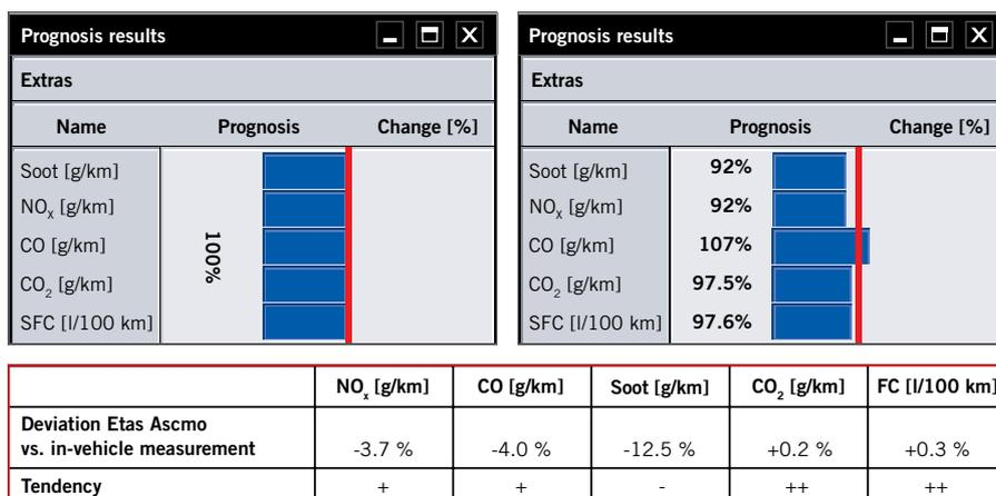
FIGURE 5 Prognosis based on cycle extrapolations before and after optimisation (partly screenshot)
