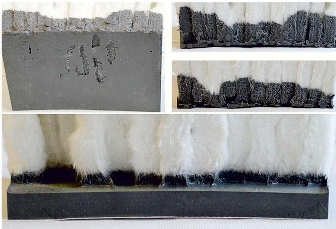
FIGURE 5 Examples of bonding tests
