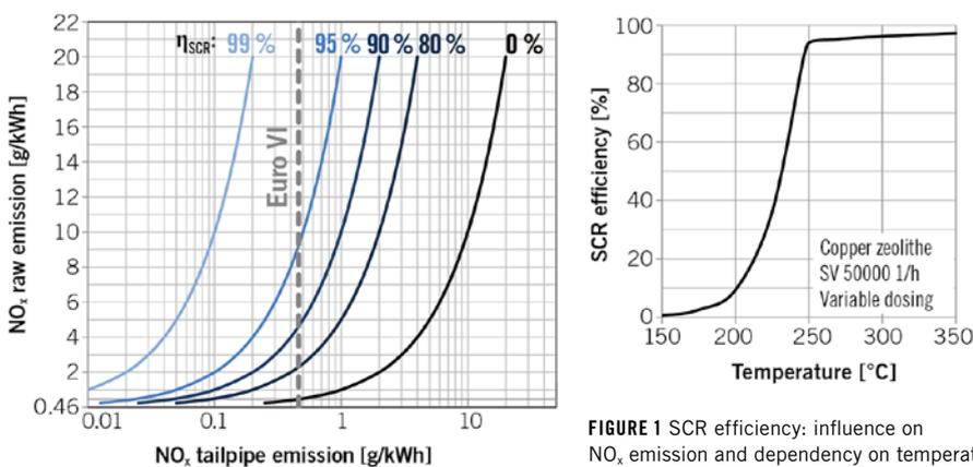
**FIGURE 1** SCR efficiency: influence on NO<sub>x</sub> emission and dependency on temperature
