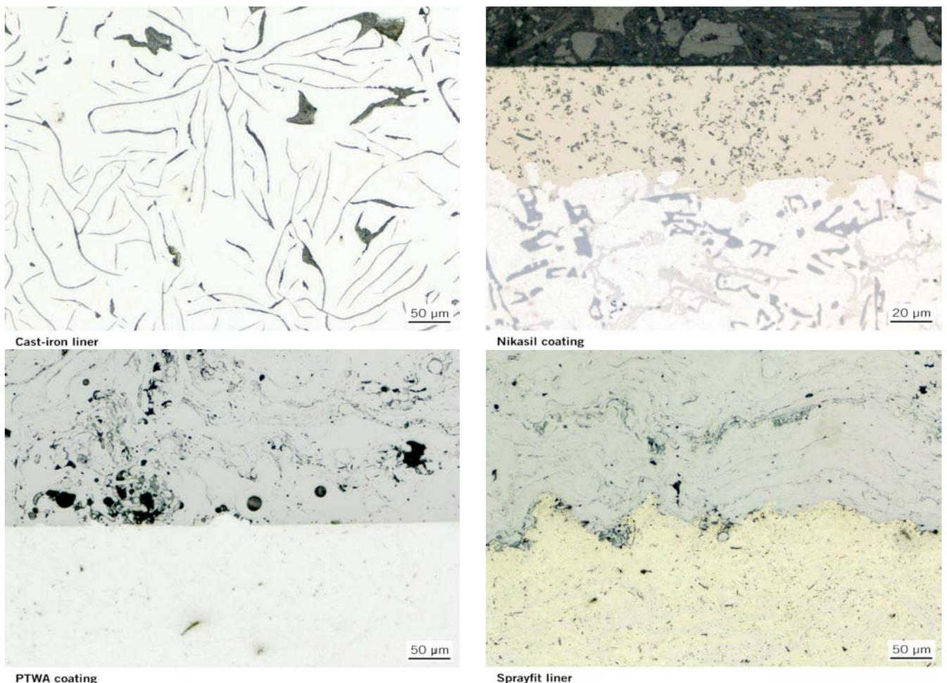
**FIGURE 1** Overview of common running surface technologies for lightweight engines
