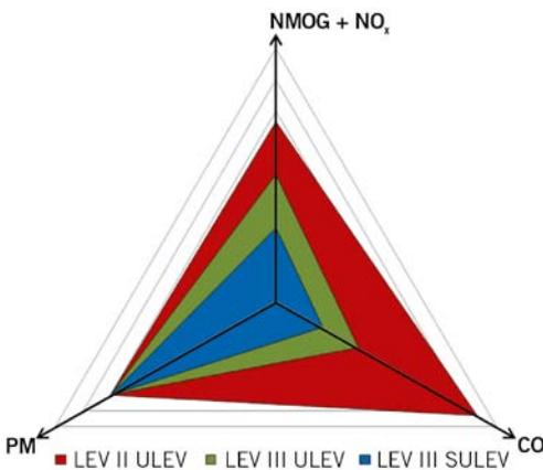
**FIGURE 5** Tightening of emission standards since LEV II
