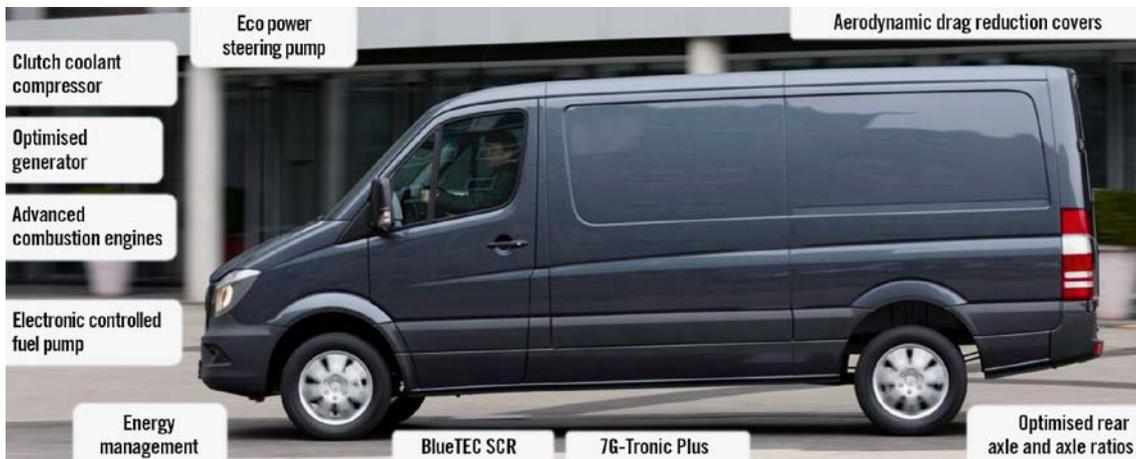
FIGURE 3 Efficiency features to improve fuel economy and CO<sub>2</sub> emissions
