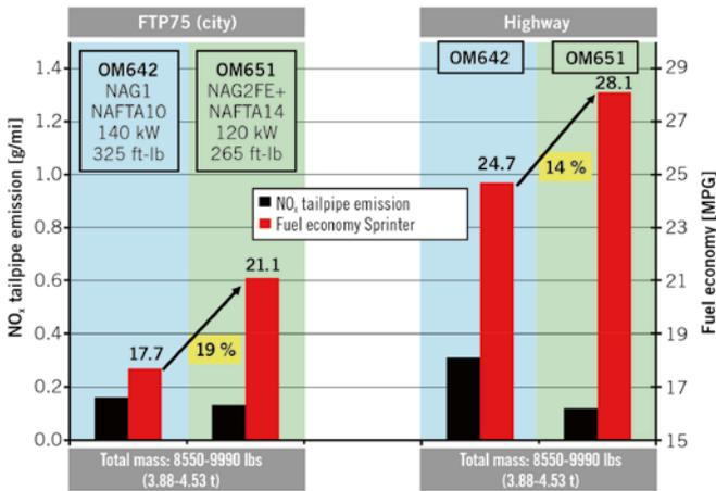
FIGURE 8 Clearly improved fuel economy and NO<sub>x</sub> emissions with OM651 Sprinter
