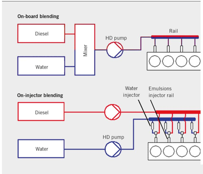
FIGURE 7 Schematic setup of on-board and on-injector blending systems
