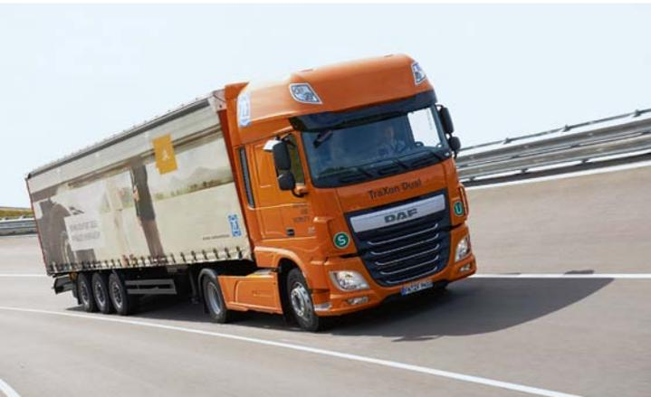
**FIGURE 5** Test vehicle from ZF with the Traxon Dual dual clutch transmission system and very high-g geared axle ratio being tested in practice
