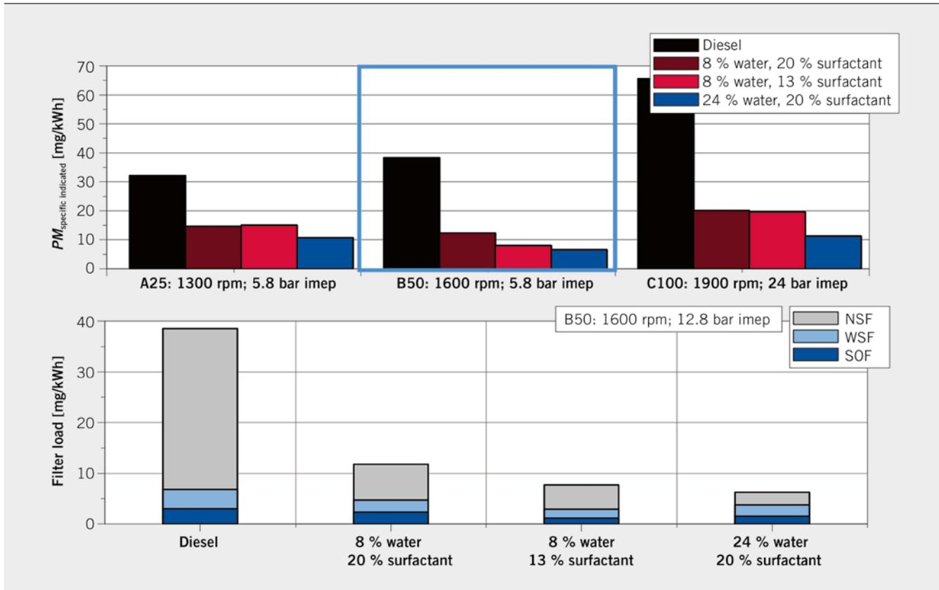
FIGURE 4 Particulate mass in examined load points and particulate composition exemplary in load point B50
