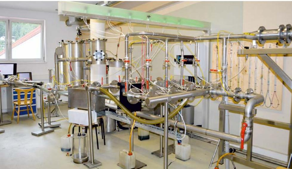
FIGURE 1 Simulation test bench for separator testing
