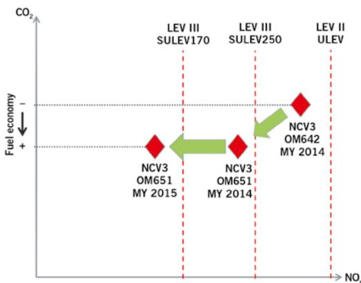
FIGURE 10 Position of SULEV variant in CO<sub>2</sub>/NO<sub>x</sub> comparison (schematically)
