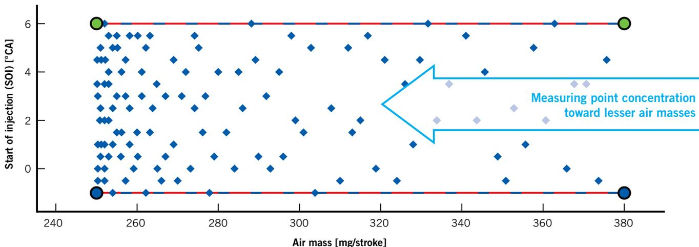
FIGURE 2 Experiment planning using local measuring point concentration
