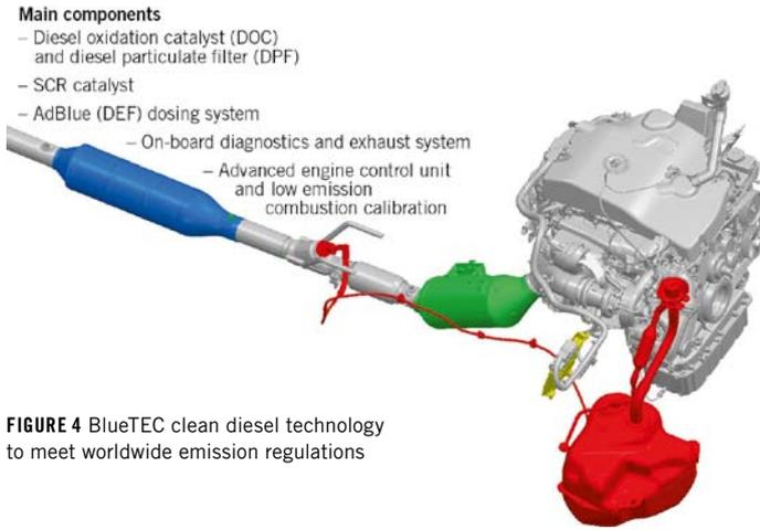
**FIGURE 4** BlueTEC clean diesel technology to meet worldwide emission regulations
