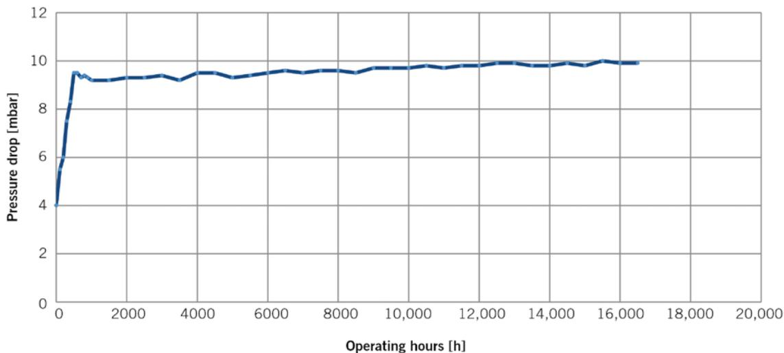
**FIGURE 3** Pressure drop trend analysis of test separator over more than 16,000 operating hours
