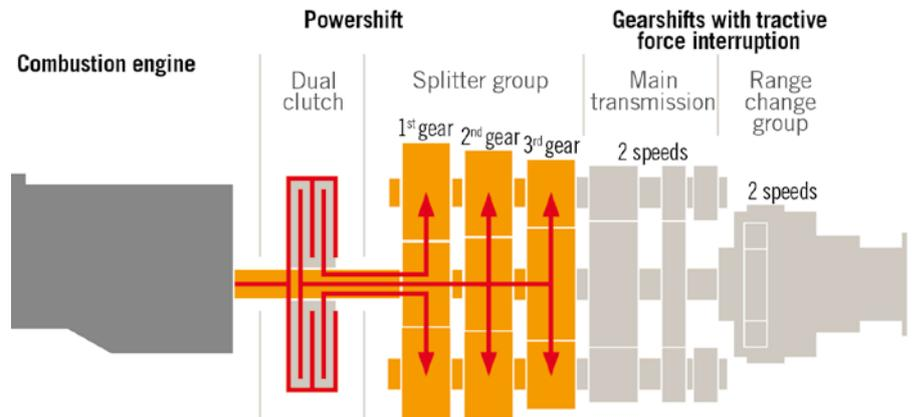
**FIGURE 2** Shift concept with dual clutch: Traxon basic transmission with splitter group, main transmission, and range change group
