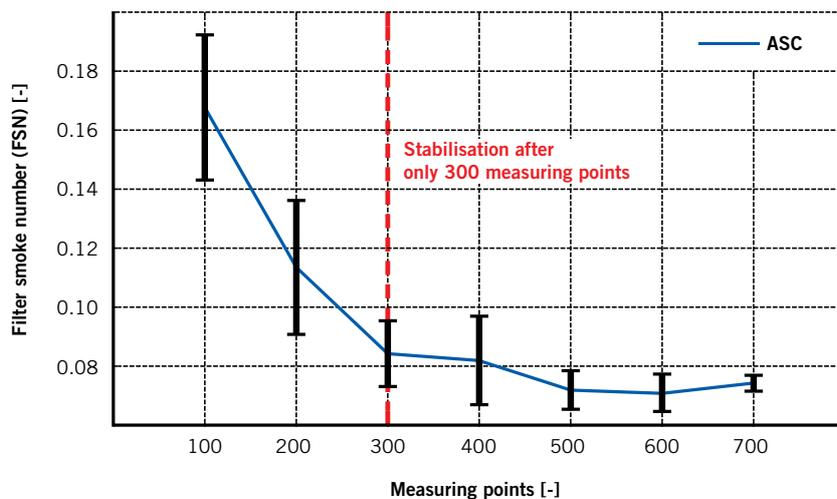
FIGURE 3 Model accuracy of Etas Ascmo model (ASC) versus data record size: mean error of global smoke number model (determined by means of verification measurements, error bar = standard deviation obtained with five repeat measurements)
