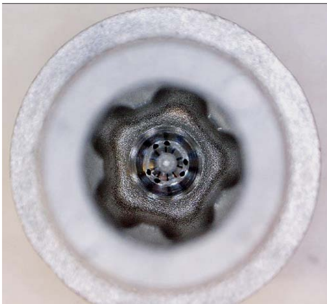
FIGURE 8 Drillings of a twin-jet prototype for testing purposes
