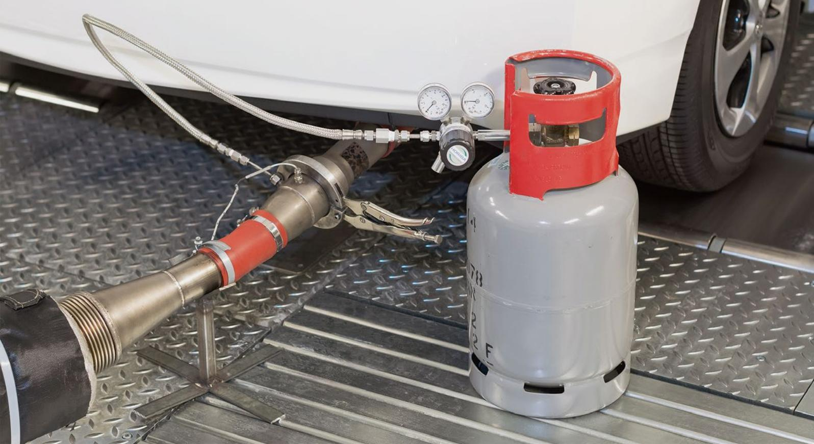
FIGURE 4 Test set-up to investigate mass transport with propane gas (© Horiba)
