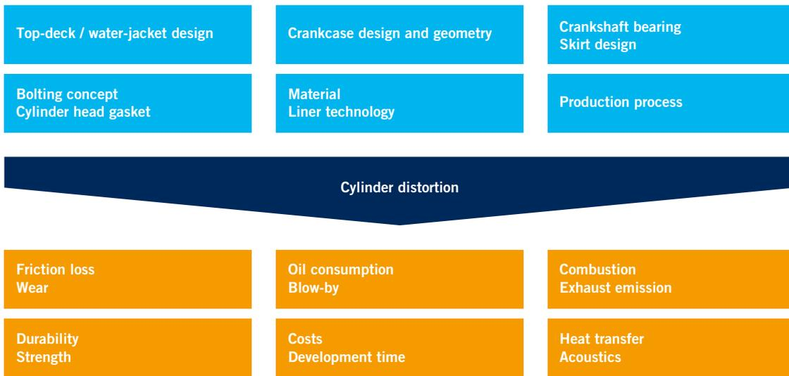
FIGURE 3 Influencing parameters and effects of cylinder distortion (© IAV)
