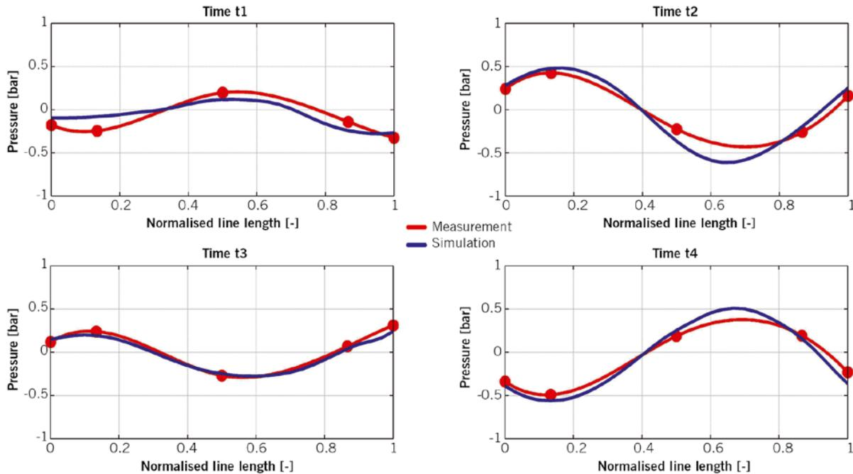
FIGURE 5 Display of the second natural frequency at about 1400 rpm (© Bosch)
