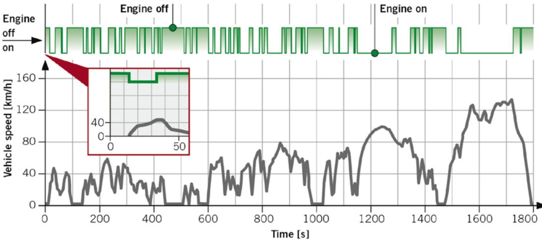
FIGURE 2 Engine-off strategy of a mid-class vehicle in the WLTC with enlarged detail of the first seconds (© Continental)
