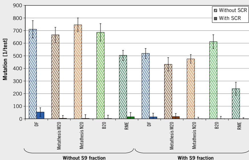
**FIGURE 7** Sum of the mutagenicity in particulate and condensate from DF and RME compared to three blend fuels at the OM 904 LA in the ETC test with the bacterial strain TA98 (© Thünen Institute of Agricultural Technology)
