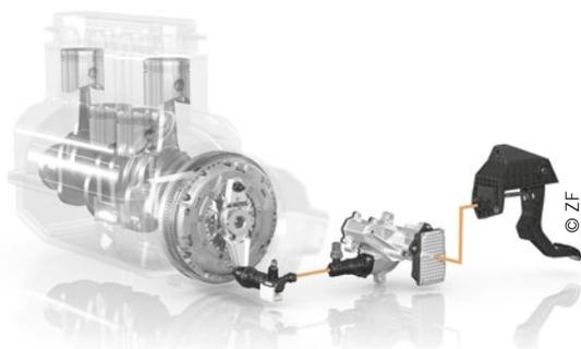
Clutch-by-Wire from ZF means important functions previously reserved for automatic transmission and automated gearboxes are now possible with manual gearboxes for the first time.
