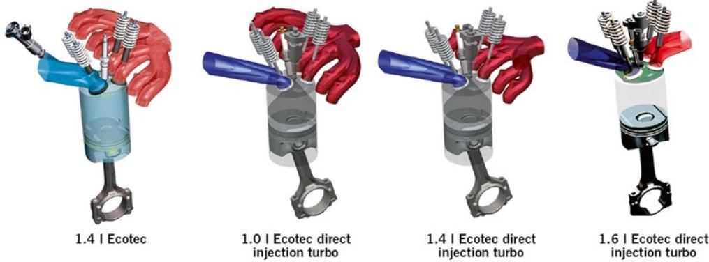
**FIGURE 5** Combustion chambers, injection and channels of the individual gasoline engines (© Opel)
