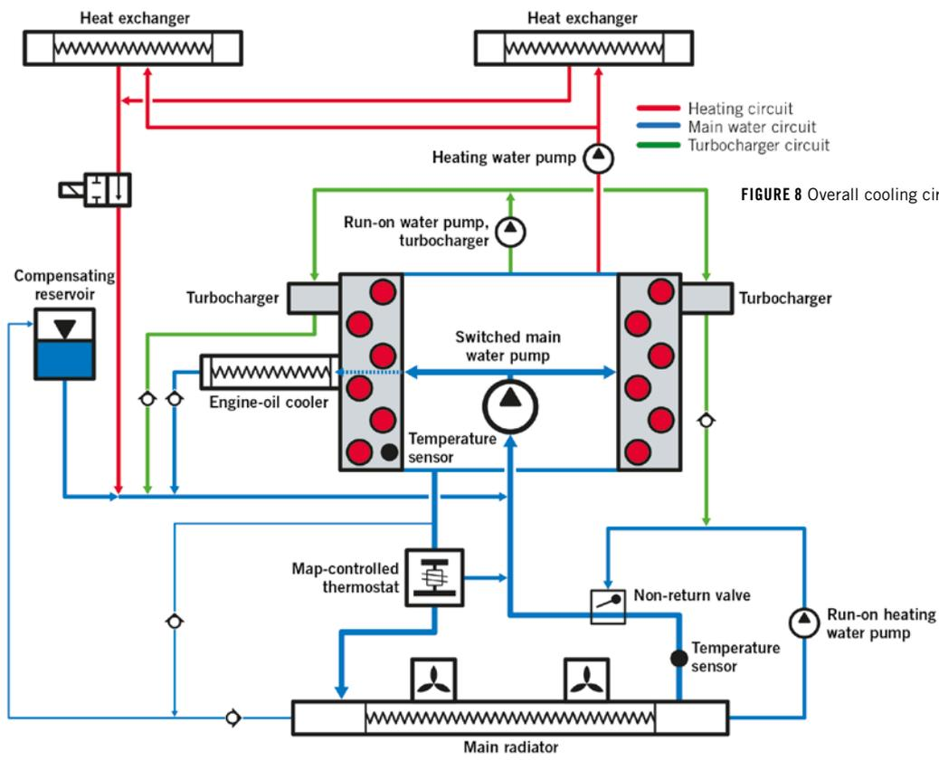
FIGURE 8 Overall cooling circuit (© Volkswagen)
