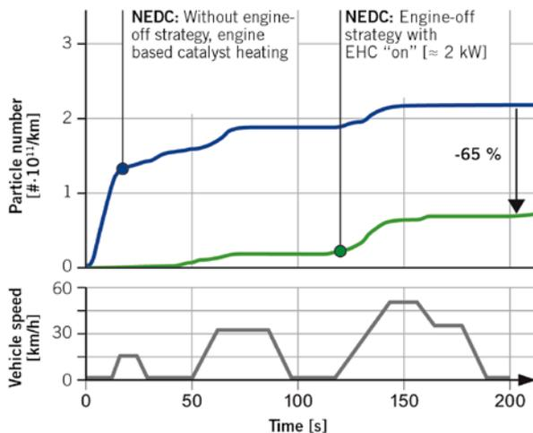
**FIGURE 5** Particulate emissions during the first 200 s in the NEDC (© Continental)
