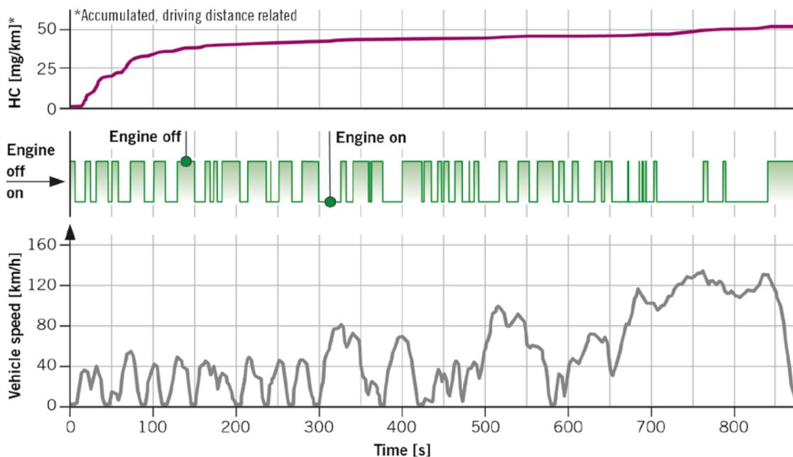
FIGURE 7 HC conversion in the RDE<sub>max</sub> driving cycle with Emicat assistance (© Continental)
