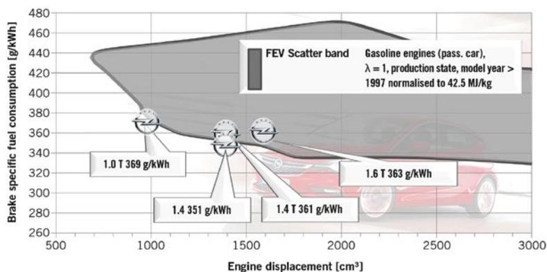
FIGURE 8 Fuel consumption of gasoline engines in the standard point 2000 rpm and 2 bar BMEP (© Opel)
