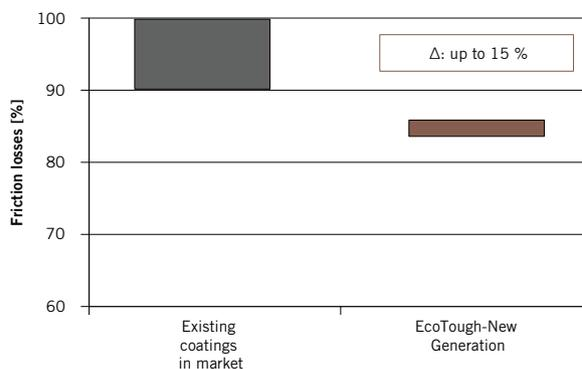
**FIGURE 2** Wear and friction of the EcoTough-New Generation skirt coating for gasoline engines as compared to the market standard (© Federal-Mogul)
