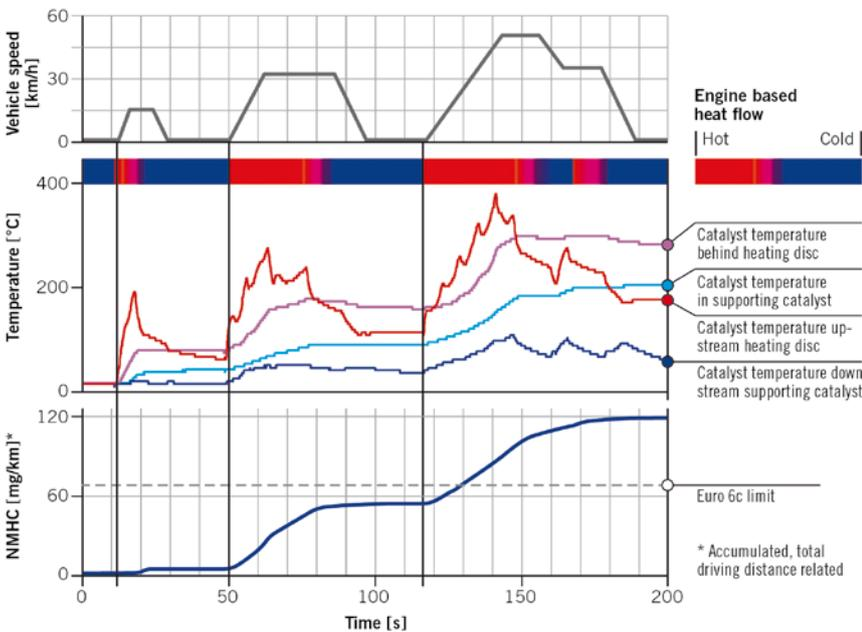
FIGURE 4 NMHC emission behaviour with a consistent engine-off strategy with Emicat compared with a conventional catalyst (© Continental)
