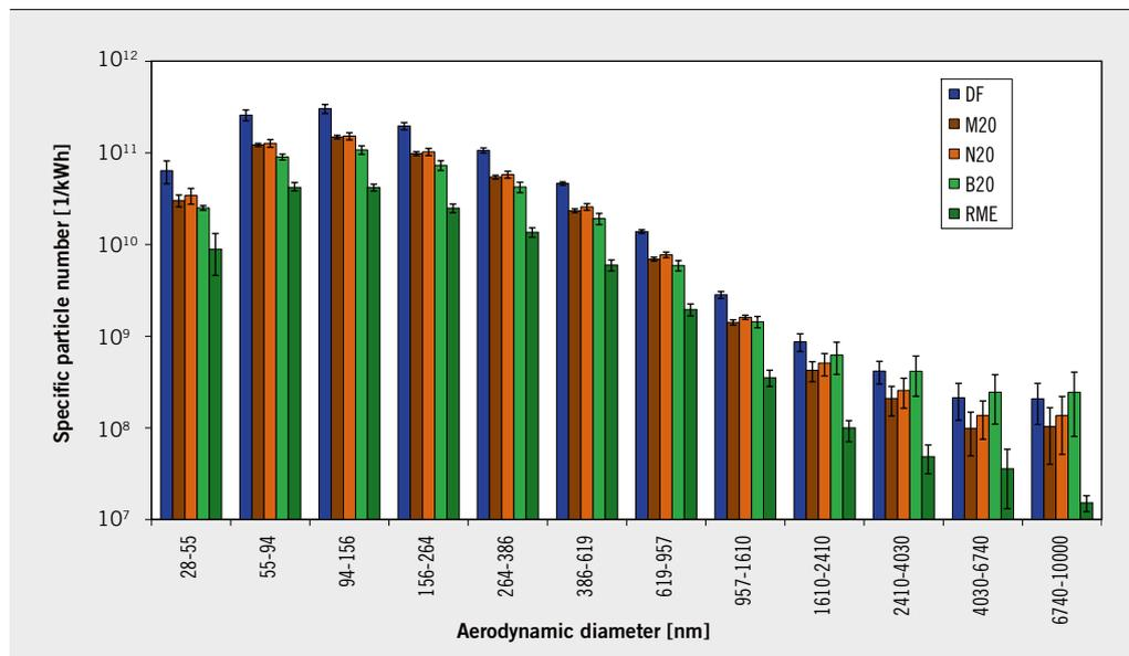
**FIGURE 5** Particle size distribution of fossil diesel fuel, 20 % blends of both metathesis fuels and biodiesel in DF, and neat biodiesel, tested in an OM 904 engine with SCR catalyst (ETC test) (© Thünen Institute of Agricultural Technology)
