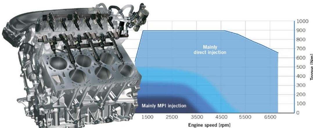
**FIGURE 3** Engine mapping for direct and MPI injection when the engine is warm (© Volkswagen)
