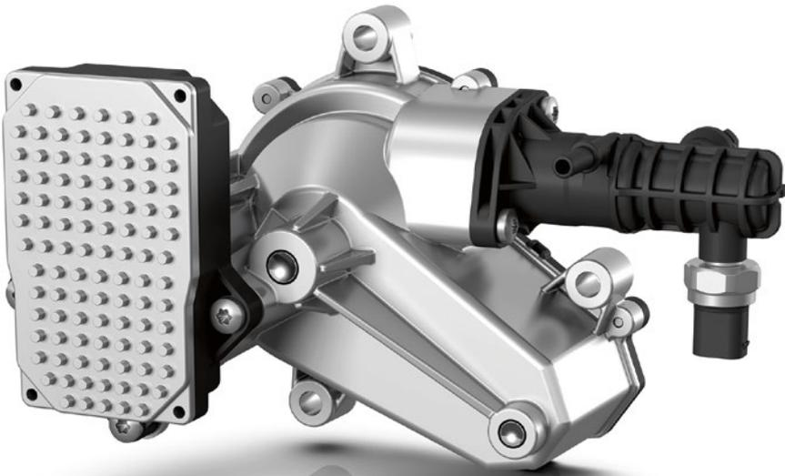
FIGURE 2 Electrohydraulic CBW actuator inclusive master cylinder for hydraulic applications, EC engine, and clutch control unit (© ZF)
