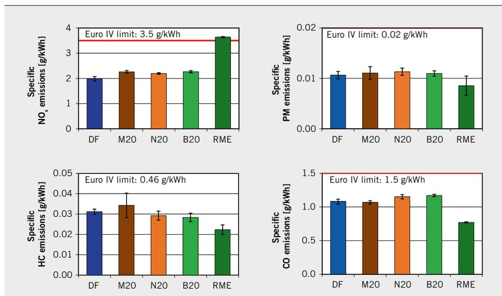
**FIGURE 4** Emission of fossil diesel fuel, 20 % blends of both metathesis fuels and biodiesel in DF, and neat biodiesel, tested in an OM 904 engine with SCR catalyst (ETC test) (© Thünen Institute of Agricultural Technology)
