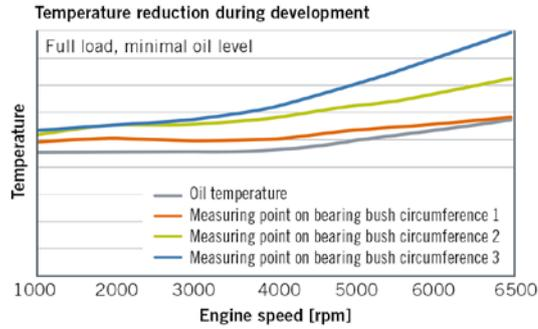
**FIGURE 2** Temperature of the bearing bushes, schematic (© Volkswagen)
