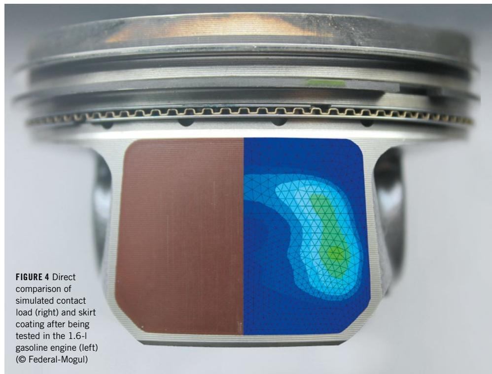
**FIGURE 4** Direct comparison of simulated contact load (right) and skirt coating after being tested in the 1.6-l gasoline engine (left) (© Federal-Mogul)
