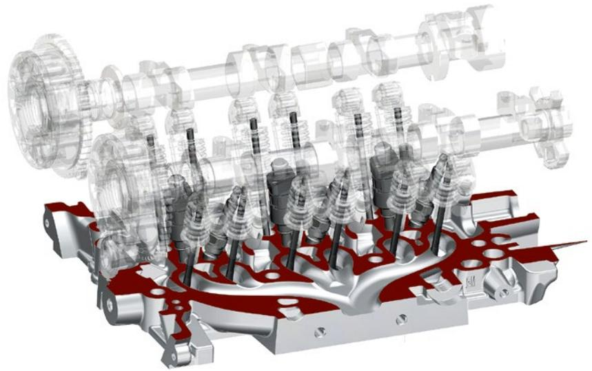
**FIGURE 4** Cylinder head with roller cam follower valve train and integrated exhaust manifold (© Opel)
