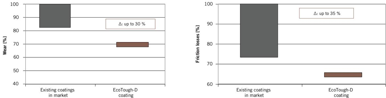
**FIGURE 6** Wear and friction of the EcoTough-D skirt coating for diesel pistons, as compared to conventional graphite-based coatings (© Federal-Mogul)
