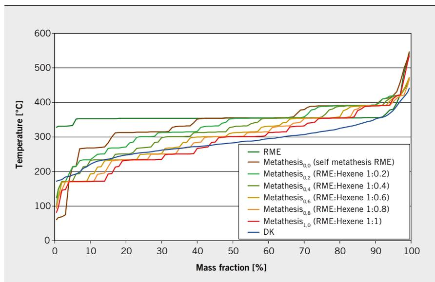
**FIGURE 3** Boiling curves of biodiesel, fossil diesel fuel and a metathesis fuel (SimDis) (© Thünen Institute of Agricultural Technology)
