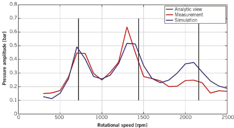
FIGURE 3 Pressure amplitude inside the low pressure line © Bosch)
