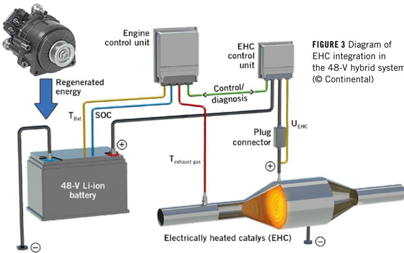
FIGURE 3 Diagram of EHC integration in the 48-V hybrid system (© Continental)
