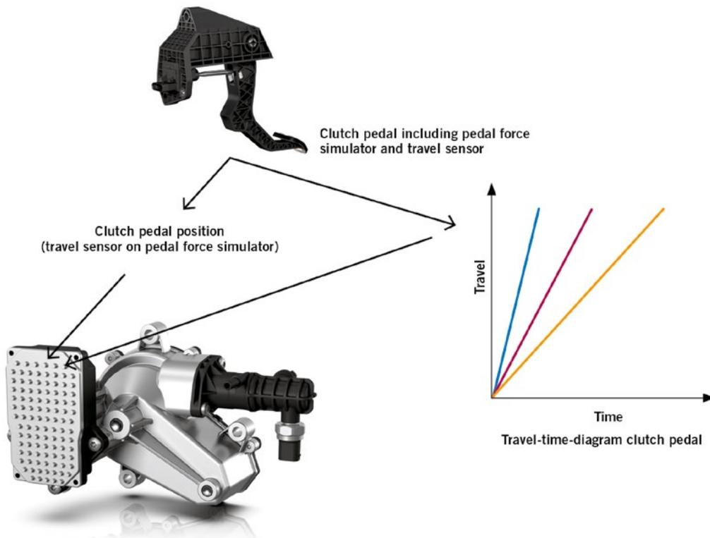
**FIGURE 4** Information transferred by the clutch pedal to the CCU, schematical (© ZF)
