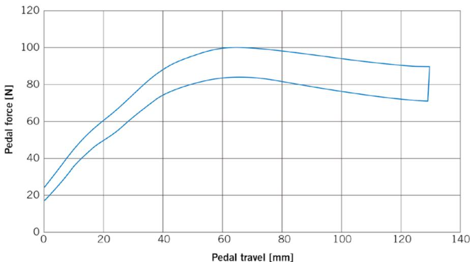
**FIGURE 5** Pedal curve of a clutch-by-wire application with a pedal force simulator for a diesel application with a maximum torque of 450 Nm (© ZF)
