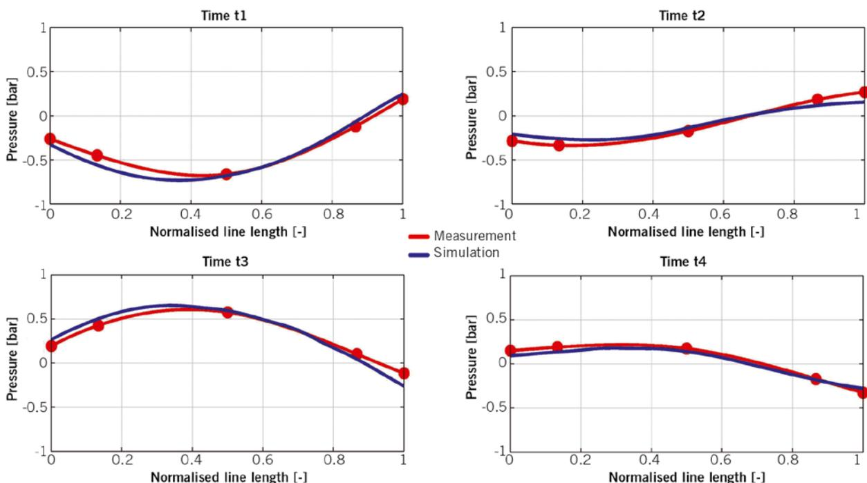
FIGURE 4 Display of the first natural frequency at about 700 rpm © Bosch)
