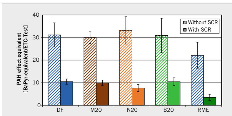
**FIGURE 6** Effect equivalent of PAH emissions from particulate and condensate of the OM 904 LA in the ETC test (© Thünen Institute of Agricultural Technology)
