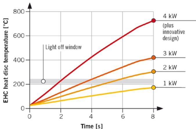
**FIGURE 8** Heat-up performance of the 9-mm-wide heating disc in the Emicat (© Continental)
