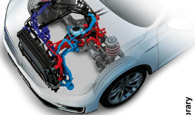
FIGURE 7 Schematic representation of three-circuit cooling system
