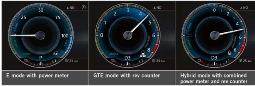
FIGURE 9 Left tube of the Active Info Display with variable read-outs
