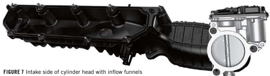
FIGURE 7 Intake side of cylinder head with inflow funnels and half-shell intake system
