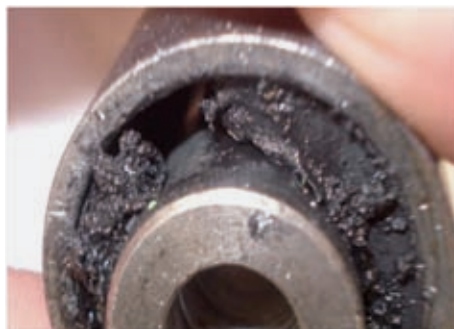
① Base mounts showing severe wear pattern (left) and objectivization of acoustic properties (right)
