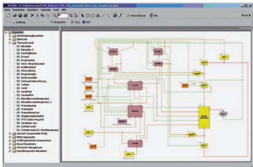
Figure 2: The cylinder module integrated in GPA. It is connected with “containers” for gas-exchange simulation and with elements for simulating the wall temperatures of cylinder liner, cylinder head, piston and valves
