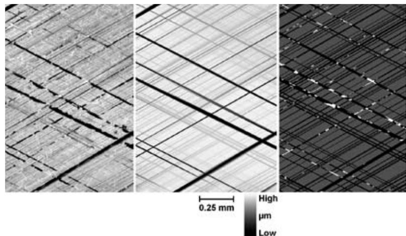
Figure 3: Sample structural separation; left: surface image excluding cylinder; center: grooving image after separation; right: relevant grooving, contact area, and sheet jacket images (binarized and superimposed)
