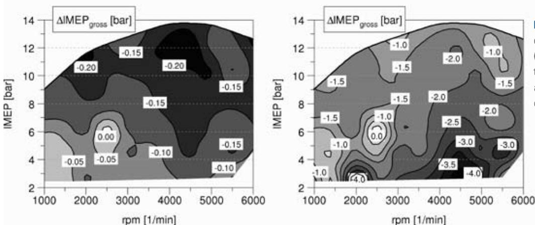
**Figure 8:** Accuracy of quasi-dimensional combustion models (passenger vehicle spark-ignition engine) for calculation with a constant parameter set in the entire engine map
