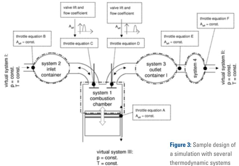
Figure 3: Sample design of a simulation with several thermodynamic systems
