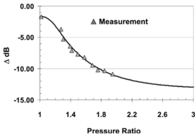
Figure 7: Attenuation behavior of a turbocharger on the intake side (load variation at 2000 rpm)
