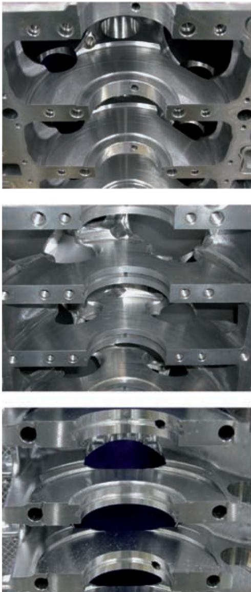
**Figure 5:** Pulsation pressure equalisation in the crankcase; drilled (above), sand-core cast (centre), milled (bottom)
