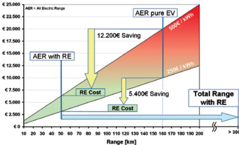
Figure 2: System cost comparison for the AVL Pure Range Extender
