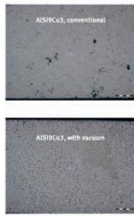
**Figure 8:** Reduction of porosity by vacuum application in high-pressure die casting; improvement of casting quality and increase in tensile strength  $R_m$  and tension/compression fatigue strength  $\sigma_{zdW}$  of high-pressure die cast bearing bulk-heads with vacuum application
