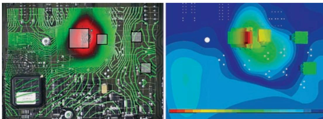
Figure 7: PCB deformation for a higher modal form – measured (left) and FEM calculation (right)
