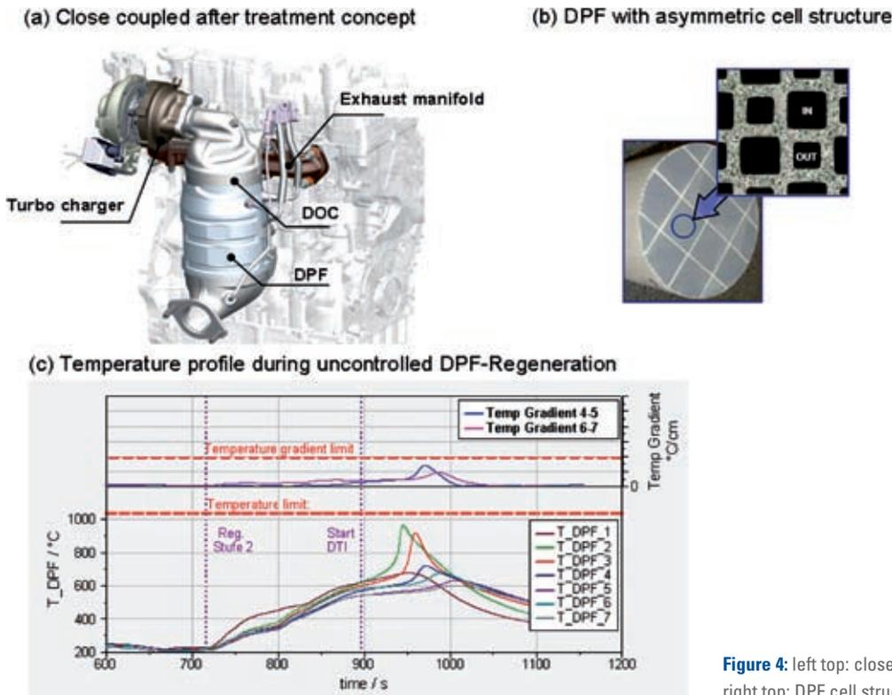
Figure 4: left top: close coupled DPF aftertreatment system; right top: DPF cell structure; bottom: temperature profile
