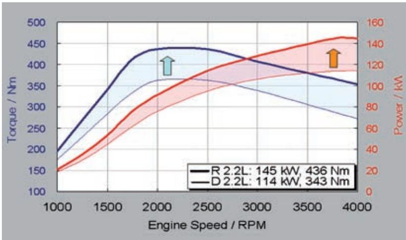
**Figure 5:** Engine power and torque at the full load conditions of the R-2.2 l in comparison to its predecessor
