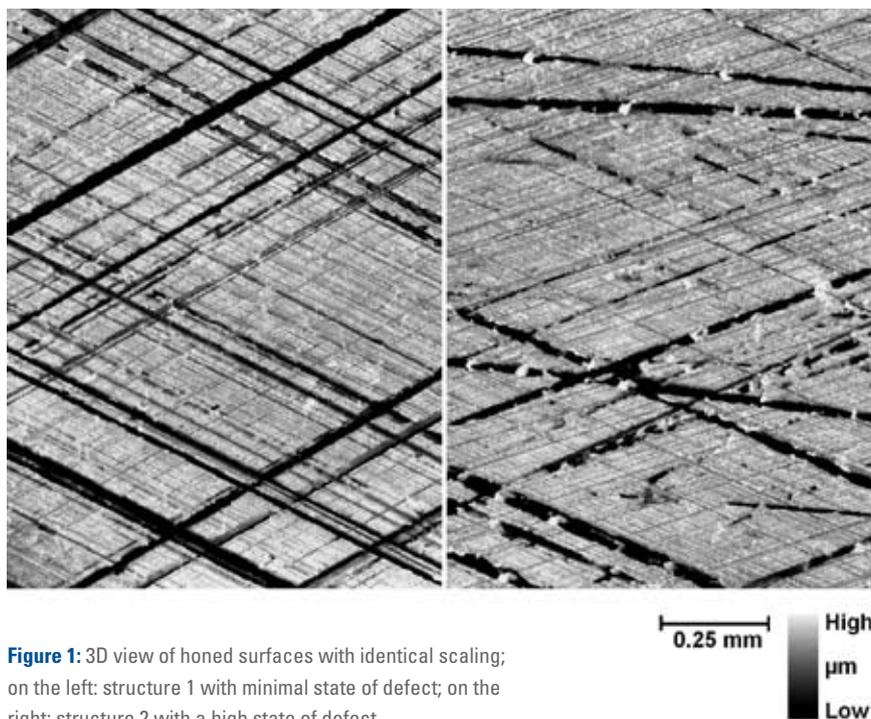
**Figure 1:** 3D view of honed surfaces with identical scaling; on the left: structure 1 with minimal state of defect; on the right: structure 2 with a high state of defect
