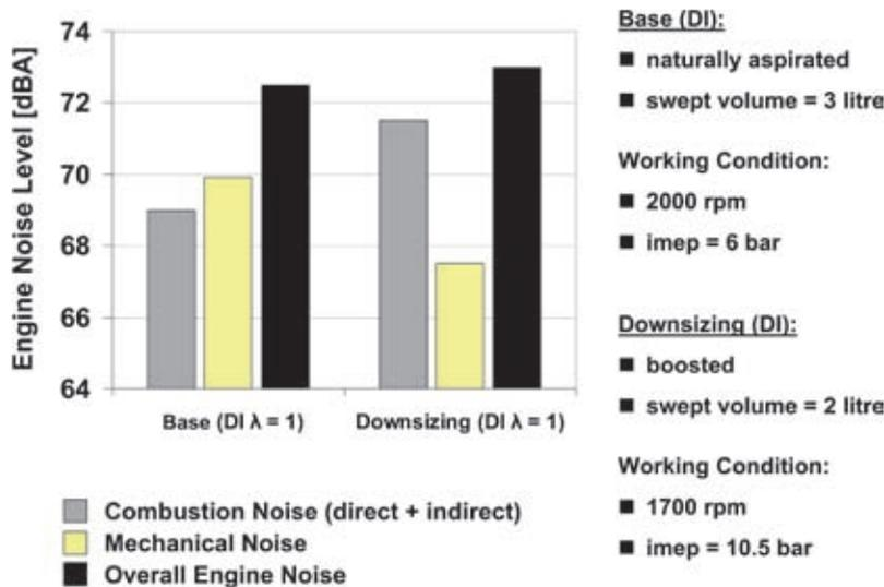
Figure 8: Noise behavior with downsizing and rpm reduction
