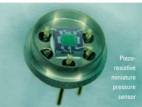
Piezo-resistive miniature pressure sensor
