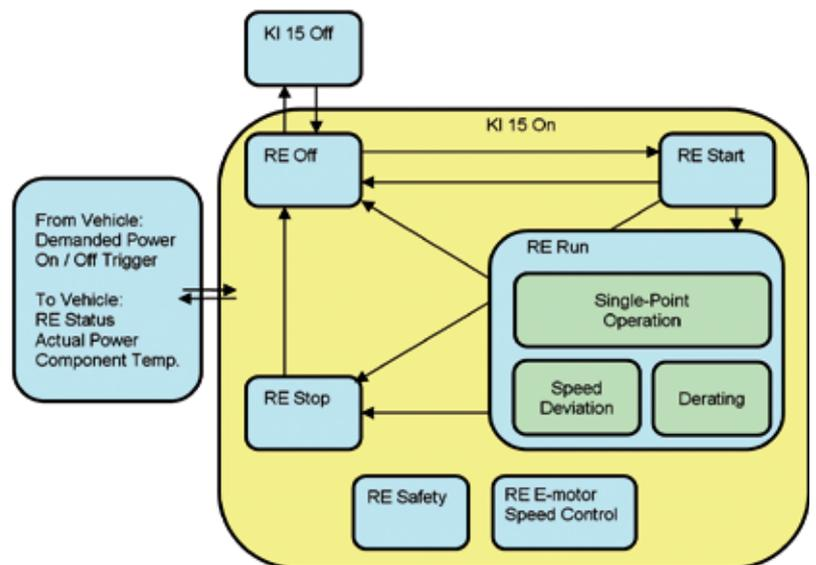
Figure 8: Concept of the system control structure
