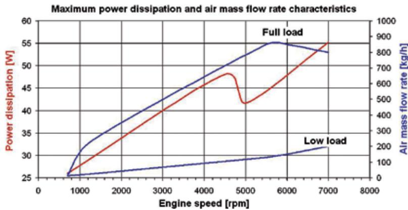
Figure 6: Relationship between air mass flow rate (load-dependent) and idealised power dissipation
