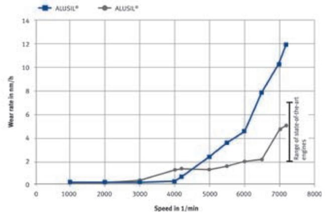
Figure 12: Strategies for the further development of ALUSIL; significant reduction of RNT wearing rate in the high-rev range
