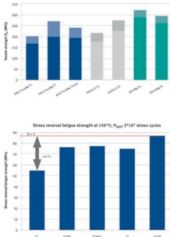
Figure 11: Tensile strengths  $R_m$  achieved with different heat treatment modes including HIP; high-pressure spraying system for casting quenching
