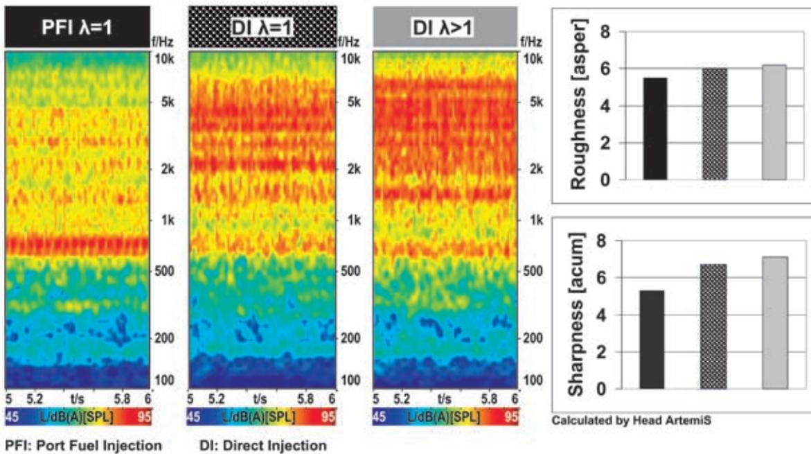
**Figure 3:** Wavelet analysis, PFI vs. DI at part load (2000 rpm, imep = 3 bar)
