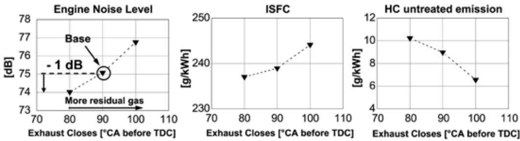
Figure 6: Parameter variation with controlled auto-ignition (2000 rpm, imep = 3 bar)
