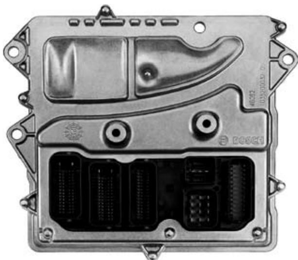
**Figure 1:** Engine control unit six-cylinder TVDI (N55)
