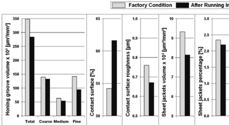
**Figure 5:** Comparison of new honing structure parameters of the surfaces, shown in Figure 4
