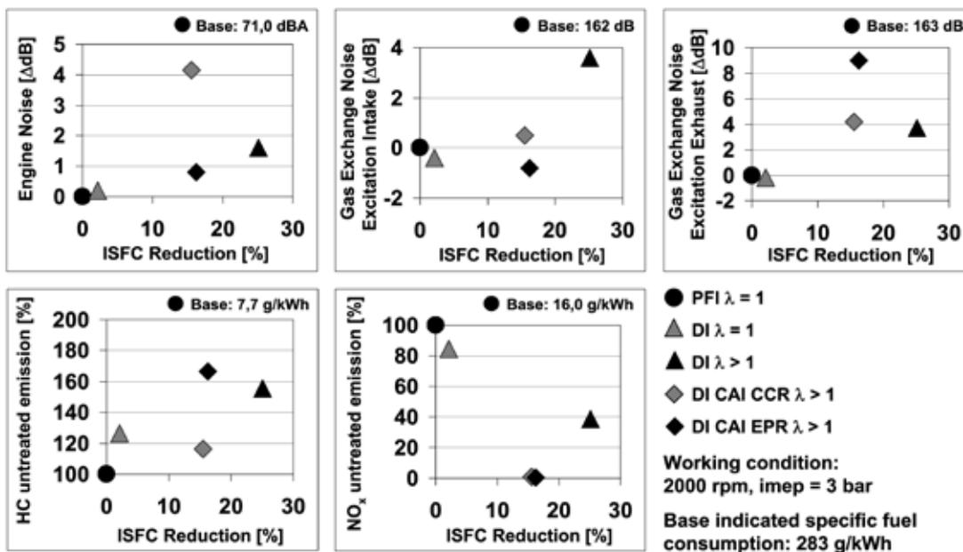
Figure 2: Noise, fuel consumption and exhaust emissions for different combustion processes at part load
