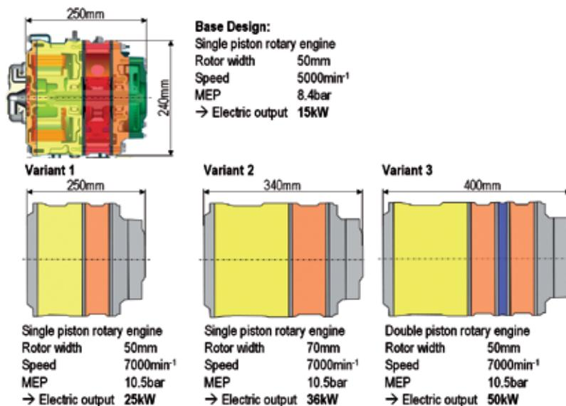
Figure 10: Performance scalability of the Range Extender core module
