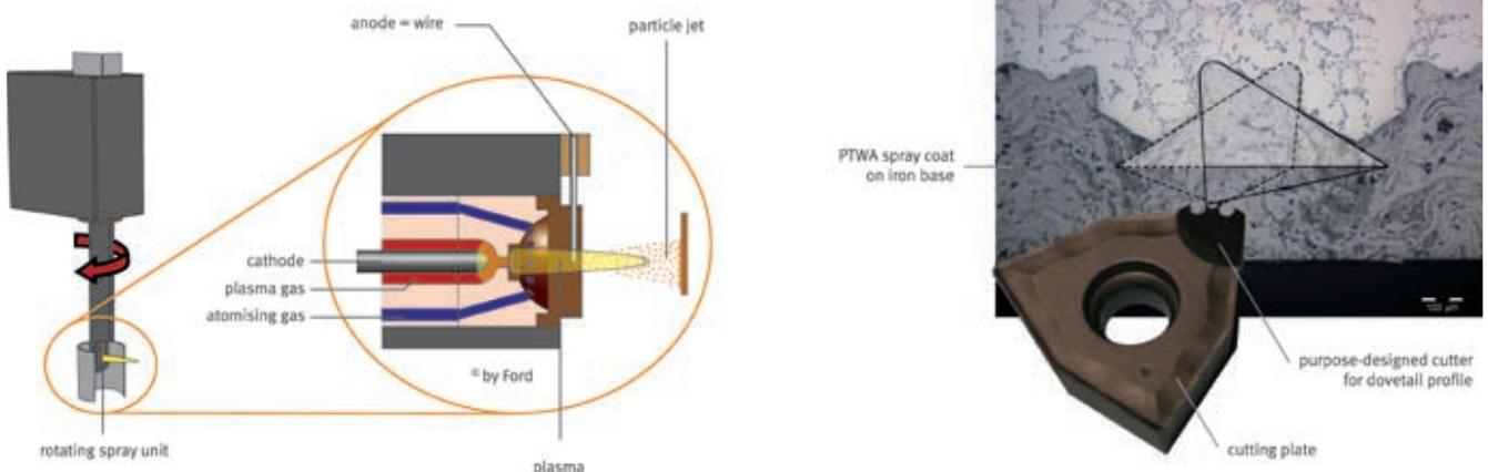
Figure 13: Principle of PTWA cylinder bore surface coating; improved coat adherence through dovetail profile
