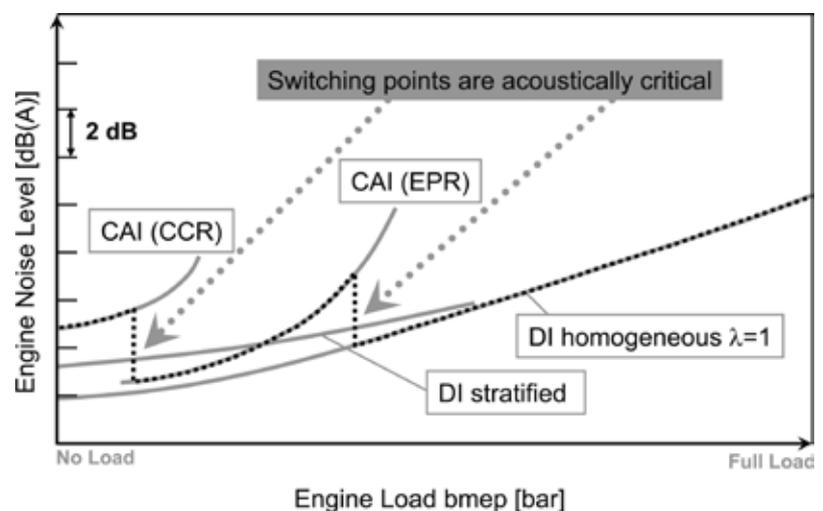
Figure 5: Process shifting problems with controlled auto-ignition (CAI)
