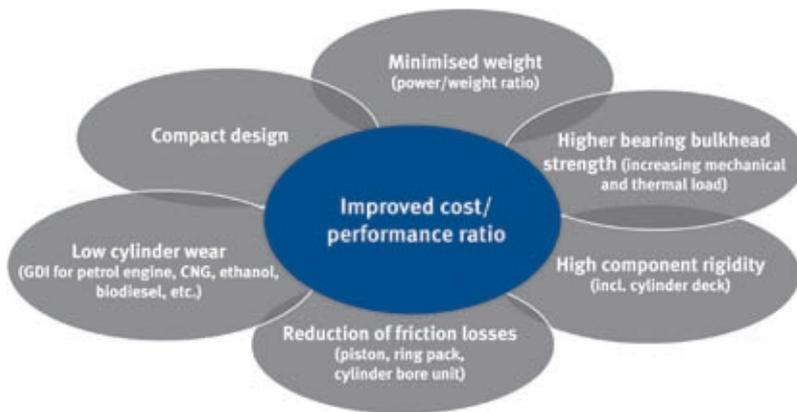
Figure 2: Challenges for cylinder block design development
