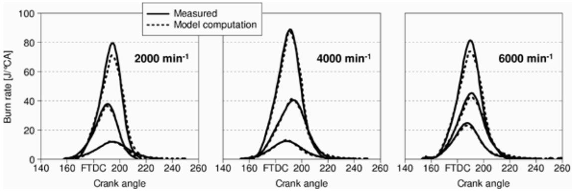
**Figure 7:** Burn rates simulated with the cylinder module (quasi-dimensional entrainment model) compared to measuring data (2000, 4000, 6000 rpm of part load to full load, passenger vehicle spark-ignition engine)
