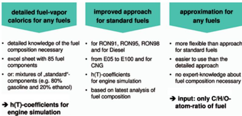
Figure 5: Approaches for calculating the fuel vapor calorics in the cylinder module
