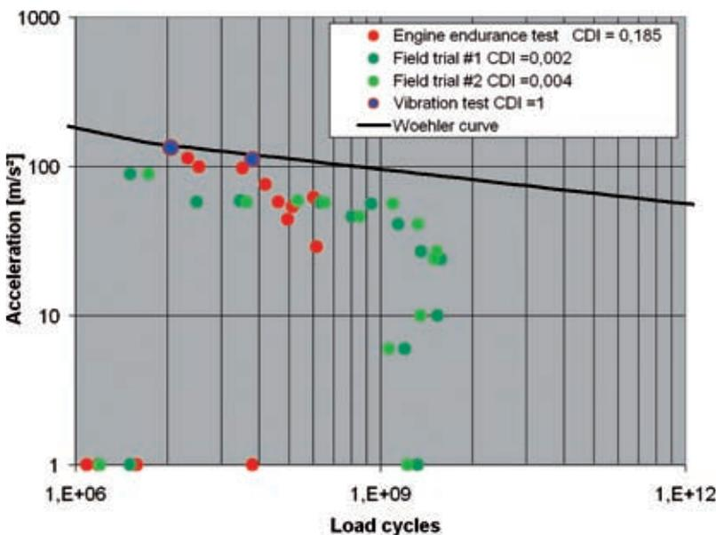
**Figure 9:** The relative damage incurred during vibration testing on the control unit is much greater than the damage incurred during endurance tests or field trials (assumptions: vibration fracture, linear accumulation of damage)
