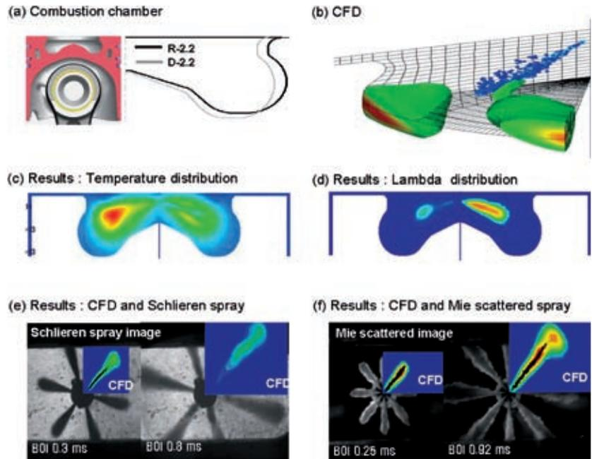
**Figure 2:** left top: combustion chamber; right top, middle, bottom: 3-D combustion simulation
