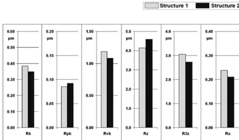
Figure 2: Contact profile parameters, determined from the profiles in Figure 1
