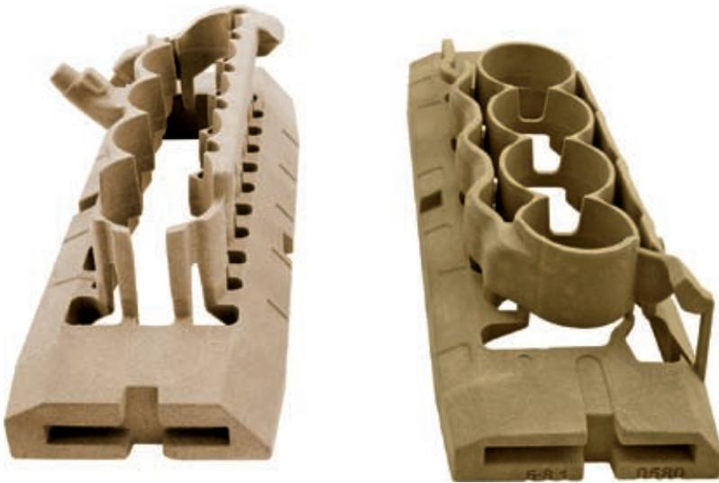
**Figure 4:** Water jacket sand cores with distribution and collector duct as well as cast cylinder land cooling
