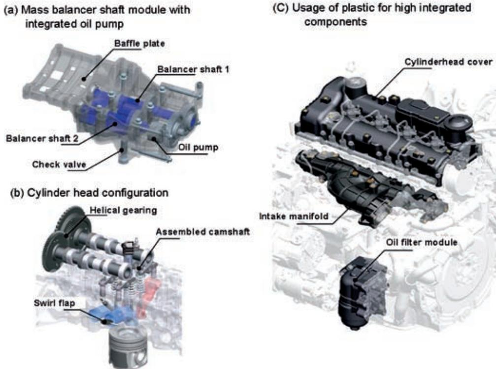
**Figure 1:** left top: mass balance shaft module; left bottom: cylinder head; right: plastic parts
