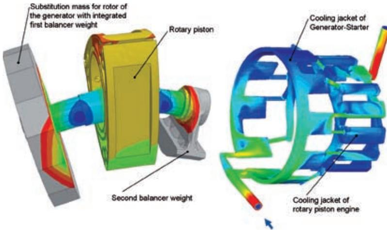
Figure 7: Simultaneous strength and CFD simulation
