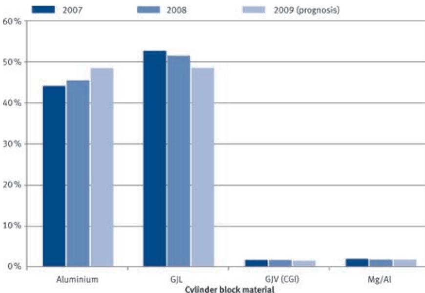
**Figure 1:** Market shares of passenger-car engines produced in Europe, according to cylinder block material
