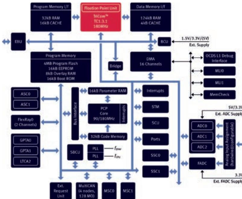
Figure 10: Architecture of the Infineon TriCore 1797
