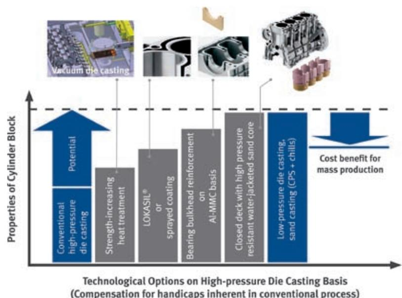
Figure 7: Concept modules of “Modular high-pressure die casting concept”
