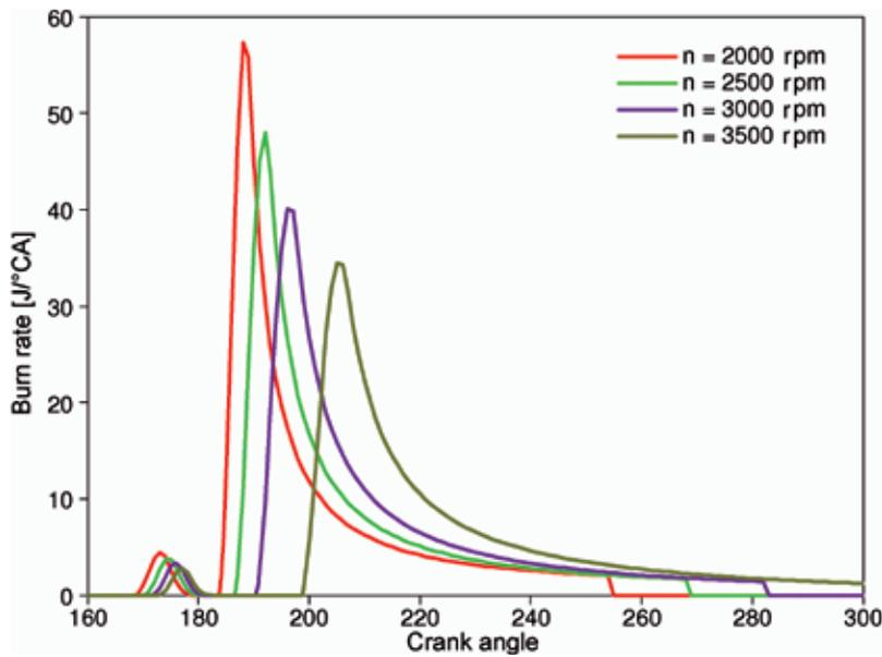
**Figure 9:** Engine speed variation with constant injection timing simulated with the Barba model (passenger car diesel engine)
