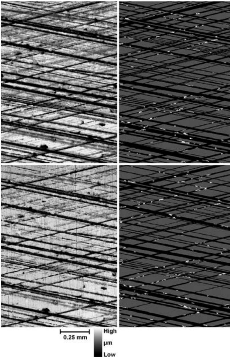
**Figure 4:** 3D View of a honed surface in factory condition (top) and after running in (bottom), at the identical position of the grooving, contact area, and sheet jacket image
