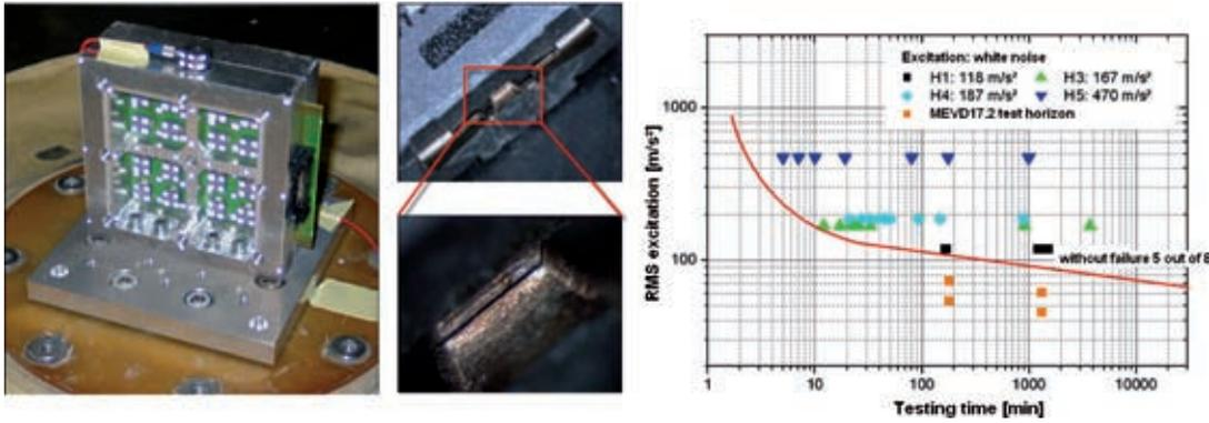
**Figure 8:** left: test structure for component testing; middle: 1. failure pattern (electrical monitoring); right: measured TTF characteristic with collective excitation and ECU test requirement
