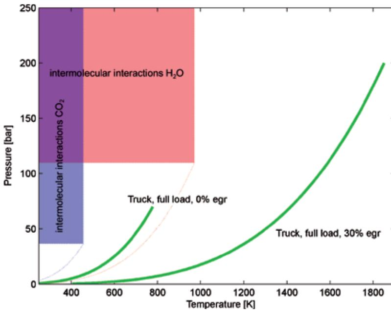
Figure 4: Temperature ranges in which intermolecular interactions in the calorics must be taken into account
