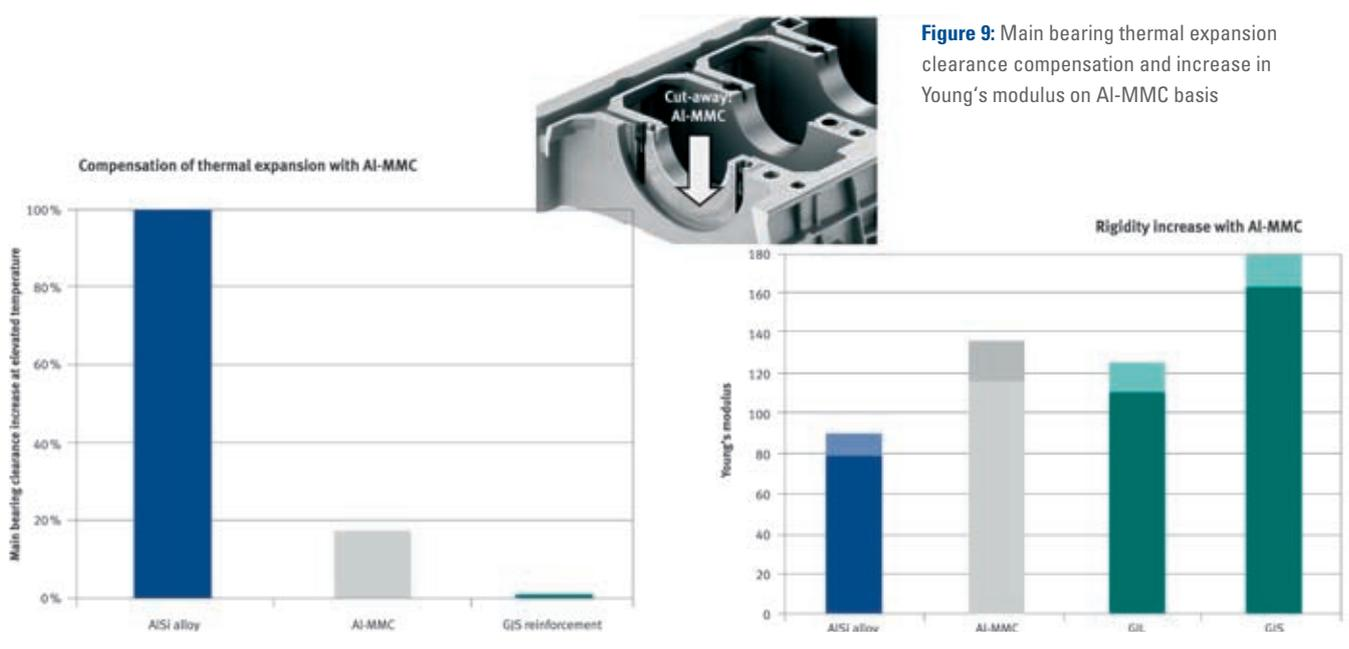
**Figure 9:** Main bearing thermal expansion clearance compensation and increase in Young's modulus on Al-MMC basis
