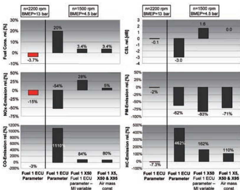
**Figure 3:** Influence of fuels on emissions in the high and low part load point and compensation measures
