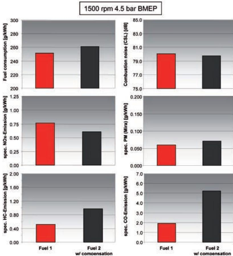
Figure 9: Emissions at a low part load point with activated fuel compensation
