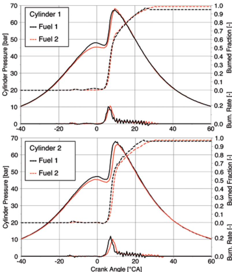
Figure 8: Comparison of combustion for different fuels with activated fuel compensation
