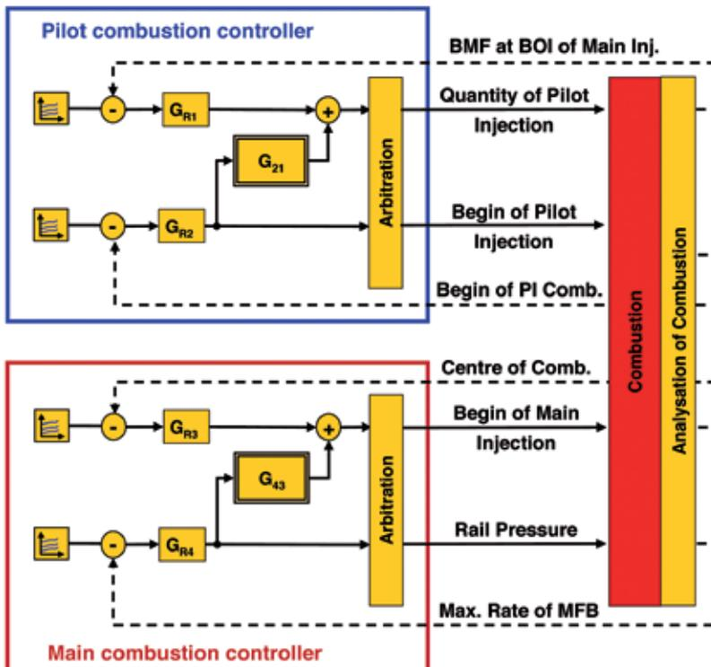
Figure 7: Control structure for fuel compensation
