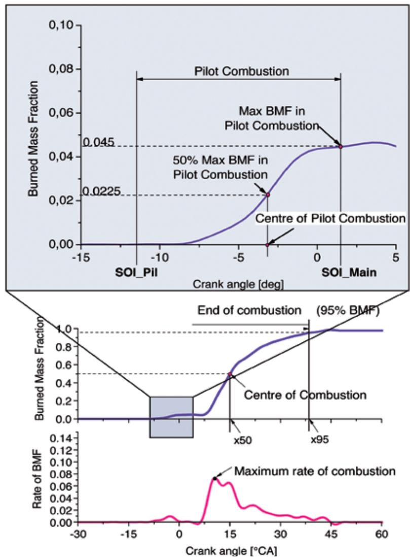
**Figure 4:** Derivation of combustion-relevant control variables
