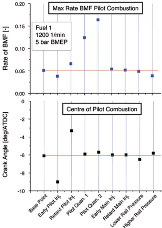
Figure 5: Influence of controlled values on pilot combustion
