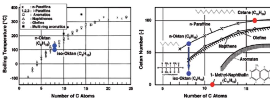
Figure 1: Some fuel properties depending on molecular structure [3]
