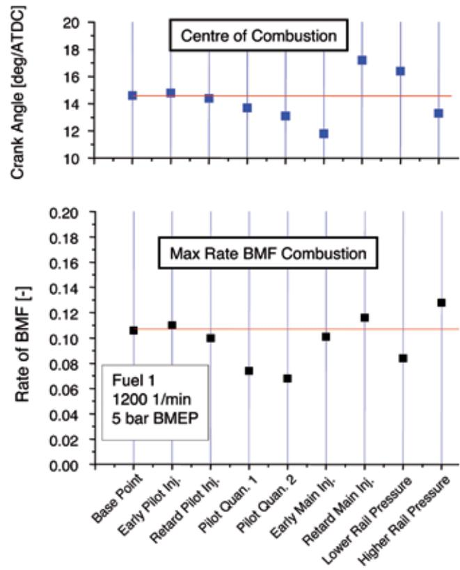
Figure 6: Influence of controlled values on main combustion
