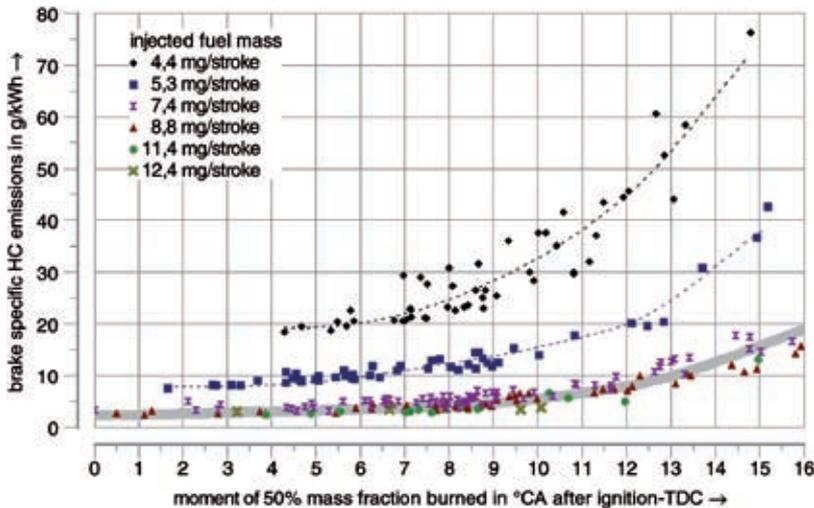
**Figure 7:** HC engine-out emissions in GCI mode depending on point of 50% mass fraction burned and injection quantity with variation of different engine setting parameters
