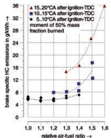
**Figure 6:** HC engine out emissions in GCI mode depending on relative air-fuel ratio and point of 50% mass fraction burned, operating point: speed 2500 rpm, brake mean effective pressure 2.0 bar, phase angle of intake camshaft varies
