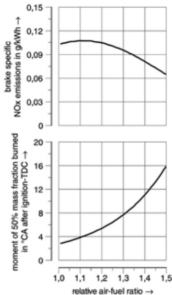
**Figure 4:** Point of 50% mass fraction burned and  $\text{NO}_x$  engine-out emissions in dependence on the relative air-fuel ratio in GCI mode, calculated from DOE data, operating point: speed 2500 rpm, brake mean effective pressure 2.0 bar
