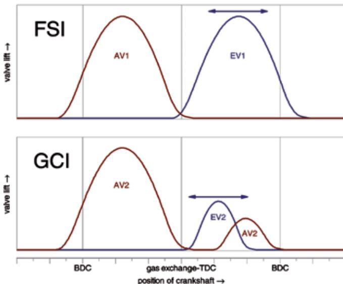
**Figure 1:** Valve lift curves in operating modes FSI and GCI
