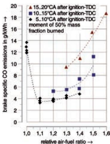
**Figure 5:** CO engine-out emissions in GCI mode depending on relative air-fuel ratio and point of 50% mass fraction burned, operating point: speed 2500 rpm, brake mean effective pressure 2.0 bar, phase angle of intake camshaft varies
