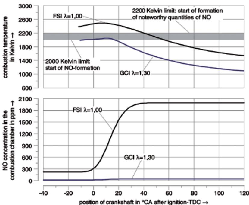
**Figure 2:** Combustion temperature and NO concentration in the combustion chamber, calculated from measured pressure curves, operating point: speed 2500 rpm, brake mean effective pressure 2.0 bar
