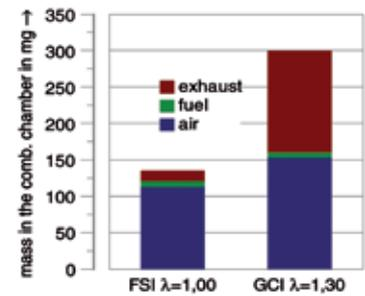
**Figure 3:** Comparison of charge composition in GCI and in FSI mode calculated from measured pressure curves, operating point: speed 2500 rpm, brake mean effective pressure 2.0 bar
