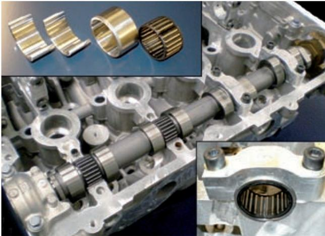
Figure 3: Cylinder head with a roller bearing supported exhaust camshaft
