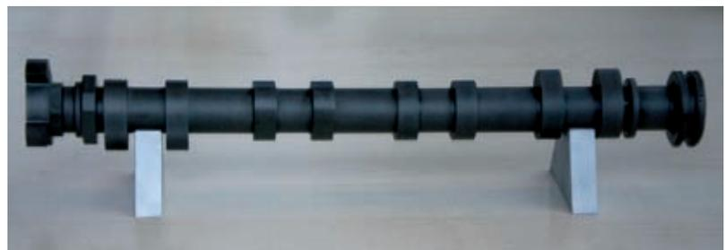
**Figure 2:** DLC-coated exhaust camshaft
