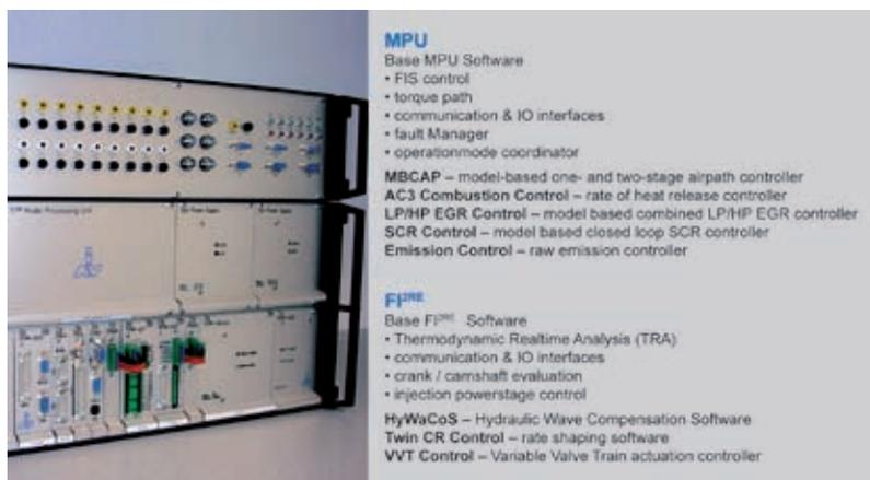
Figure 2: Modular software functions of the MPEC
