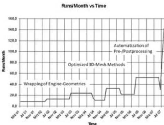
Figure 4: Increase in speed due to automatization of the CFD process
