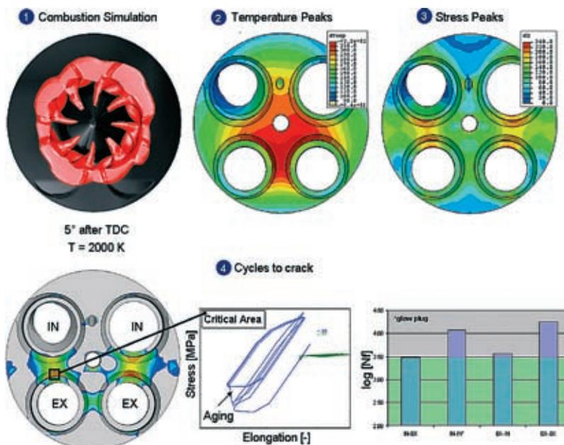
Figure 5: Crack-Simulation
