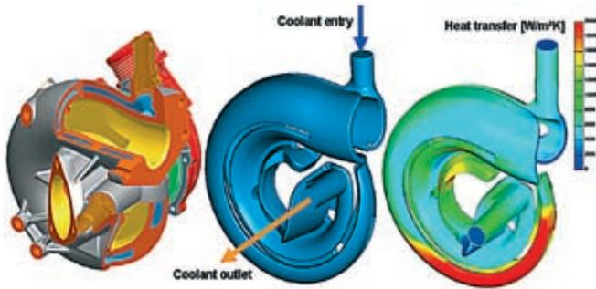
Figure 8: Water cooled aluminium VTG-Turbine
