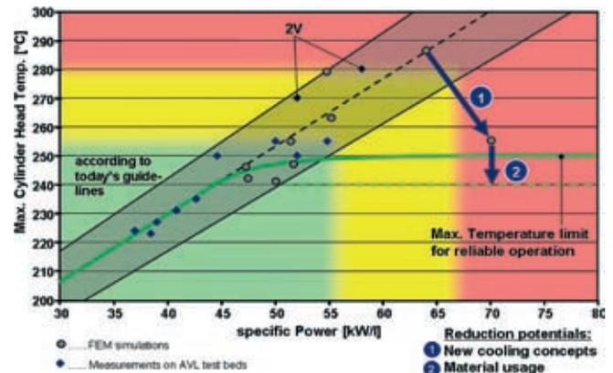
**Figure 3:** Cylinder head temperature vs. specific power
