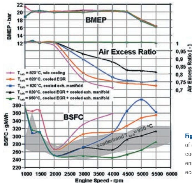
Figure 10: Influence of exhaust gas cooling on full load enrichment and fuel economy
