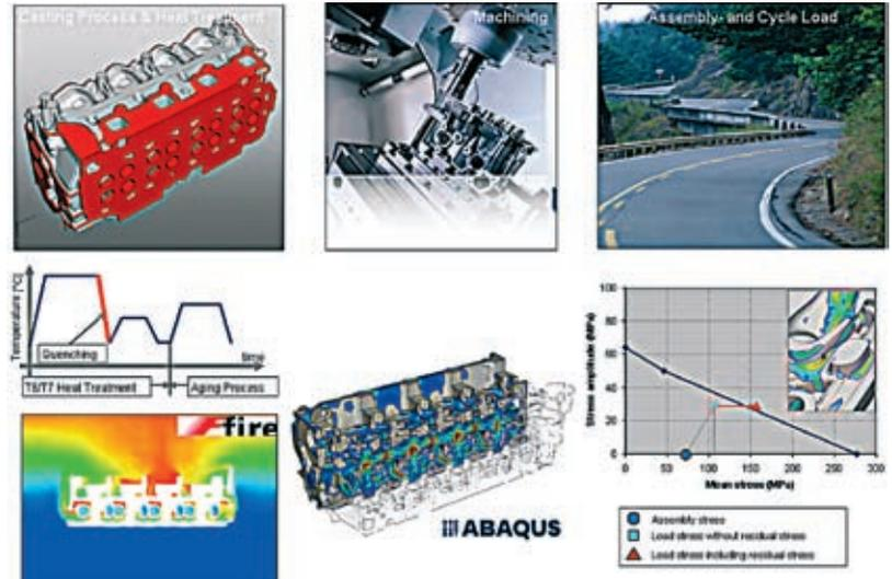
Figure 6: Stress simulation according to the manufacturing process
