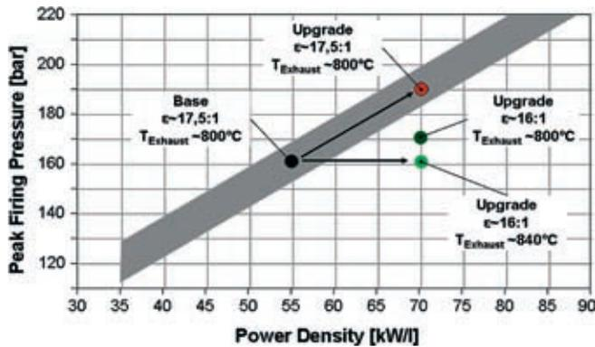
**Figure 2:** Effect of compression ratio and exhaust gas temperature on peak firing pressure
