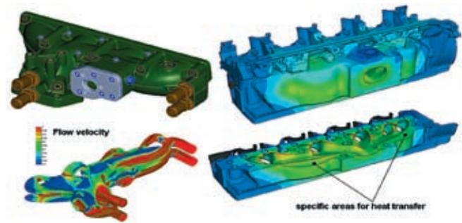
Figure 9: Cooled aluminum exhaust manifold
