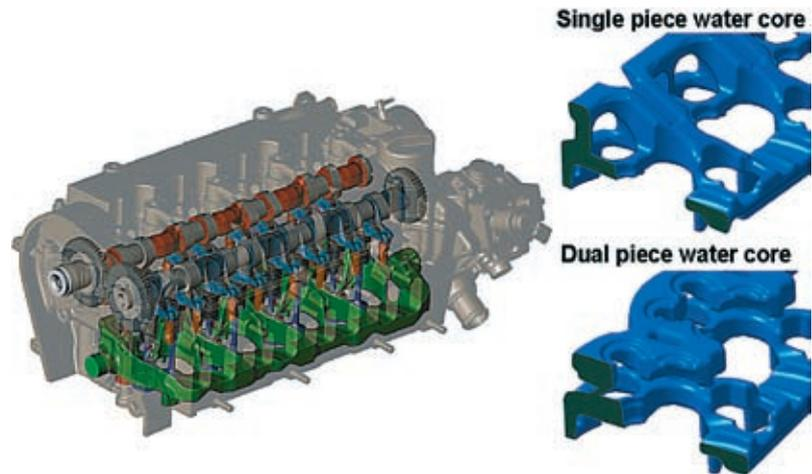
Figure 4: Crossflow cooling, single piece vs. dual piece water core
