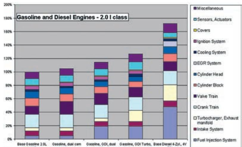
Figure 7: Technology cost comparison Gasoline and Diesel engine
