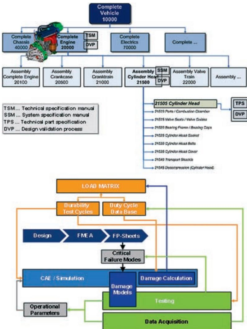
Figure 11: Design validation process (DVP) for systems, assemblies, and parts
