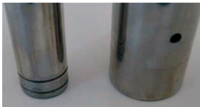
Figure 15: Polymer lapped parts after test
