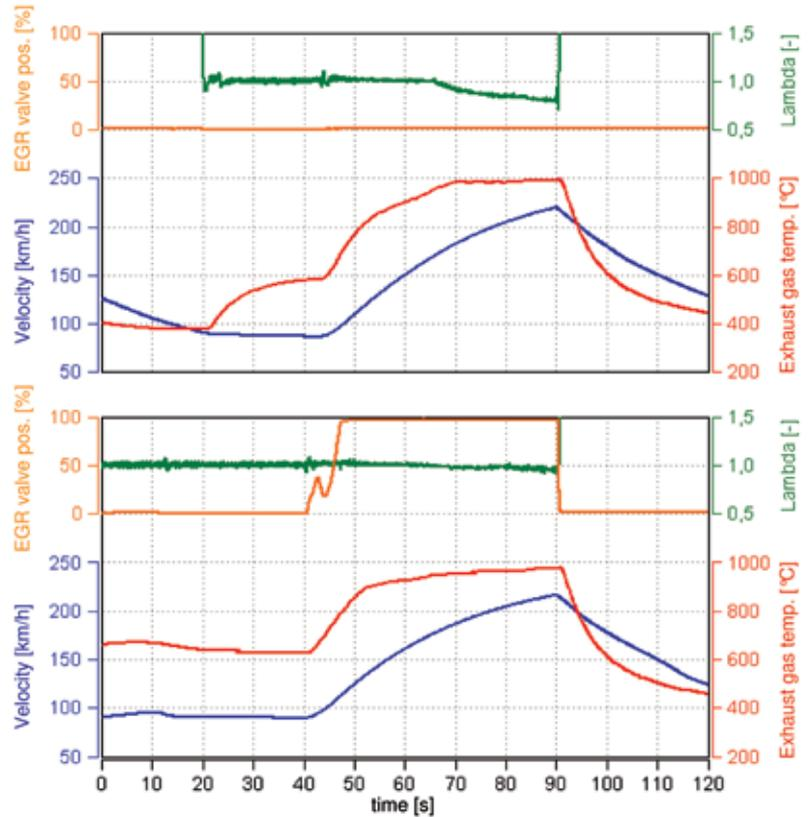
Figure 4: Vehicle acceleration in 6th gear, below with, and above without cooled EGR
