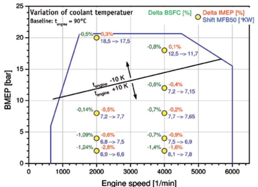
Figure 5: The effect of changes in the coolant temperature ( $t_{mot}$ ) on the combustion in the engine
