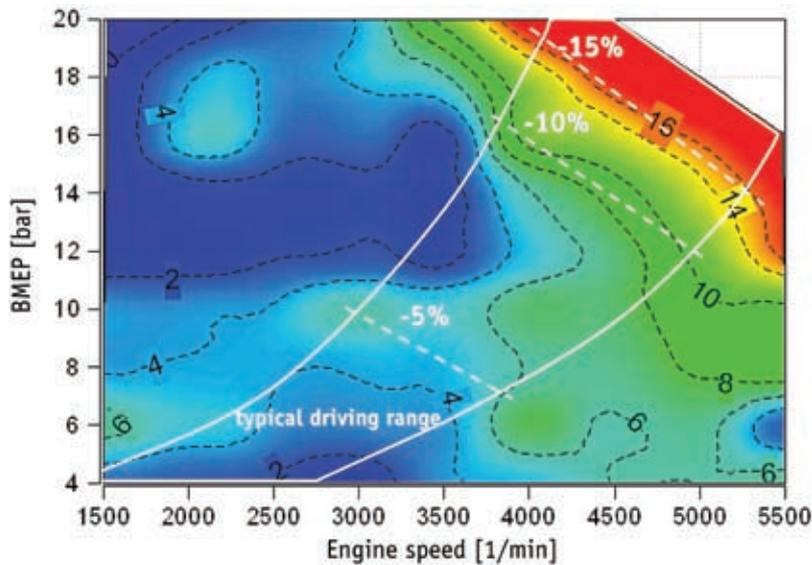
Figure 2: Map of fuel consumption reduction through the application of cooled EGR
