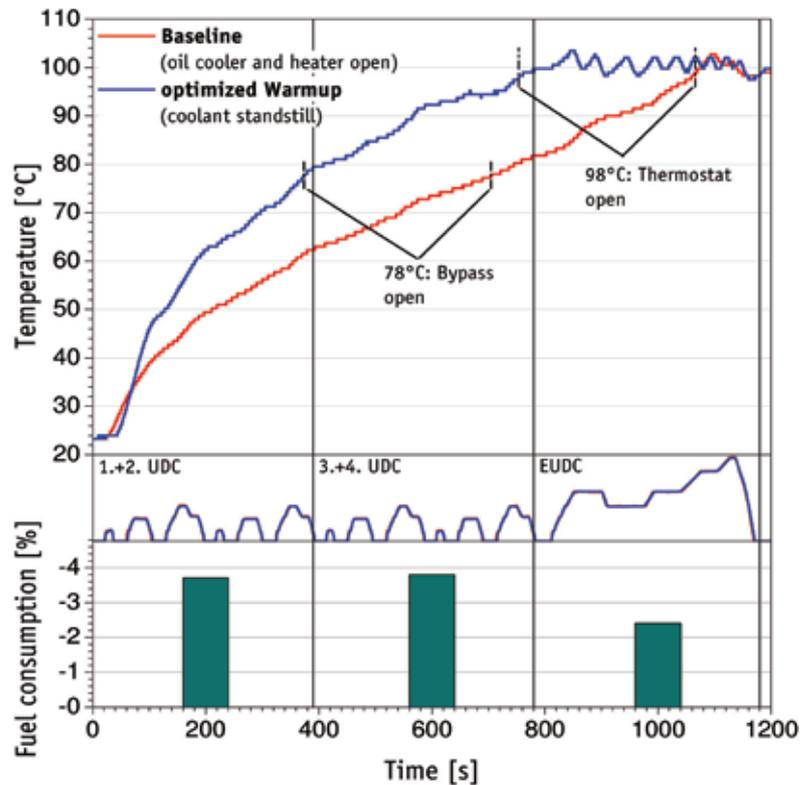
**Figure 6:** Reduction of the fuel consumption in the NEDC with the use of coolant stand still
