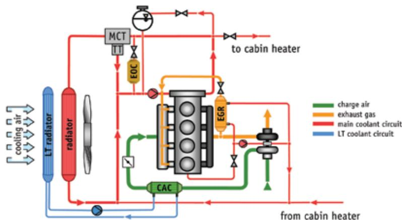
**Figure 1:** Layout of the cooling circuit
