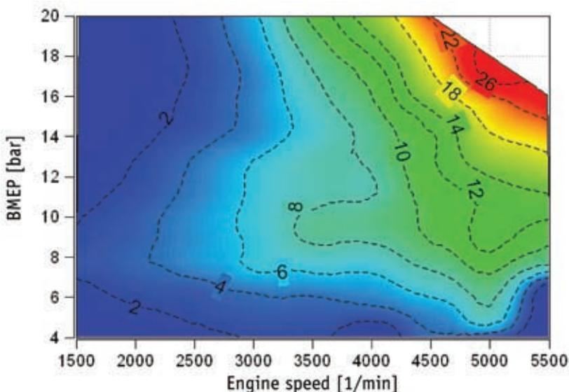
Figure 3: Heat rejection [kW] from the EGR cooler
