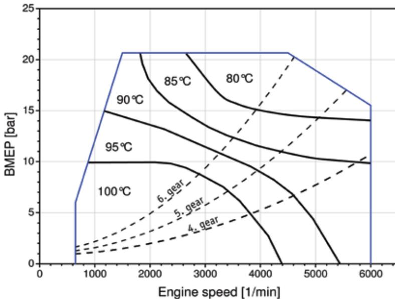
Figure 7: Coolant temperature limits across the engine map
