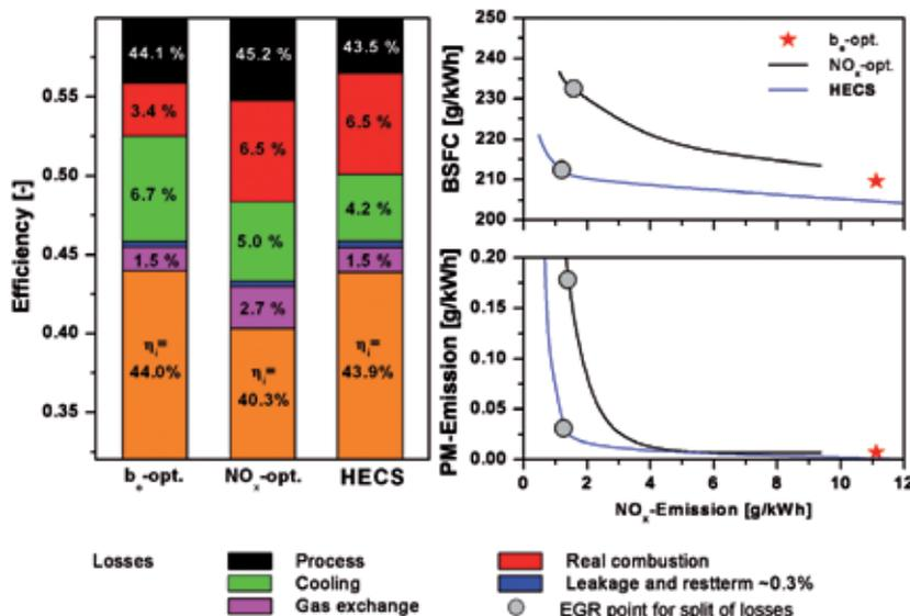
Figure 9: Break-up of losses and trade-offs at the part load point 2000 rpm,  $p_{me} = 12$  bar
