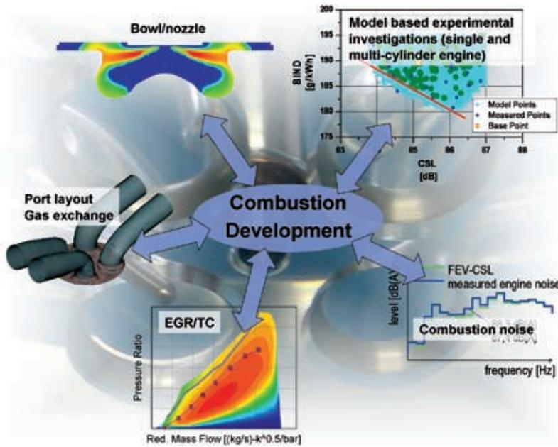
Figure 1: Tools and optimization parameters of the HECS combustion system development
