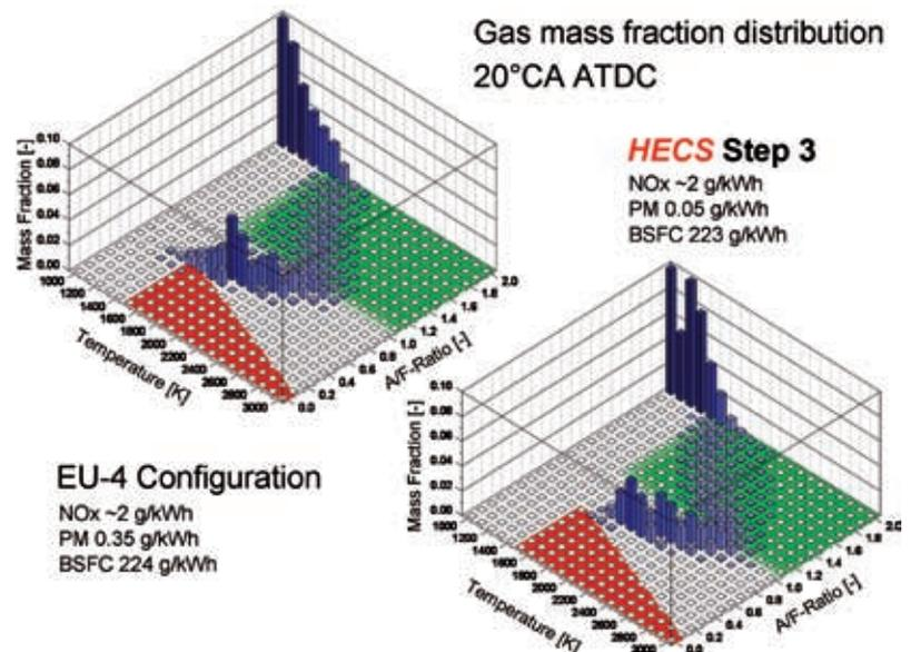
Figure 8:  $\lambda/T$  classification of the mass fractions in the combustion chamber at 20°C A after top dead centre in the Euro 4 standard and HECS combustion system, high part load
