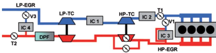
Figure 5: Schematic of the boosting and exhaust gas recirculation system that is used to meet the HECS target range for the exhaust gas recirculation rate and combustion air-fuel ratio at high loads
