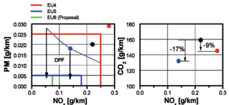
Cycle Simulation for Middle Class Vehicle (Station Wagon, 1590 kg, MT-6, 2WD)
