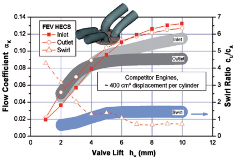
Figure 6: HECS flow characteristic and comparison to conventional processes
