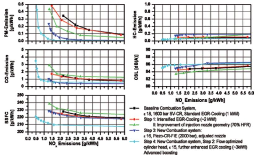
Figure 7: Evolution of the HECS combustion system at a high partial load
