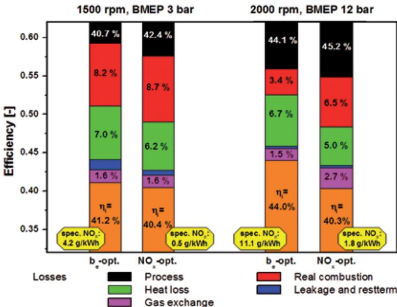
Figure 4: Break-up of losses in the part load points 1500 rpm,  $p_{me}=3$  bar and 2000 rpm,  $p_{me}=12$  bar, in each case with calibrated for minimum nitrogen oxides emissions and minimum fuel consumption
