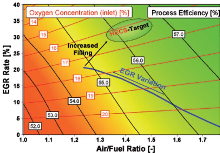
**Figure 3:** Dependence of the process efficiency on the different exhaust gas recirculation rates and combustion air-fuel ratios – 30 mg of injected fuel
