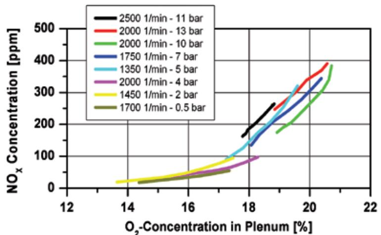
Figure 2: Dependence of the nitrogen oxide concentration on the oxygen concentration in the plenum of various, emission-relevant load points
