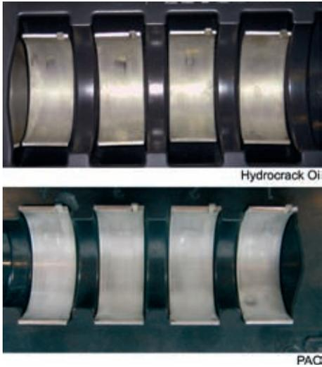
**Figure 6:** Visual appearance of connecting-rod bearing on the bearing-cover side
