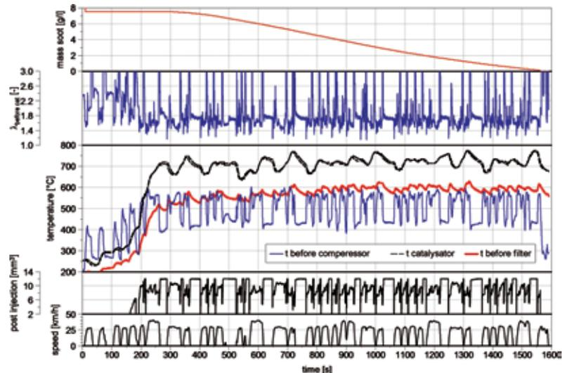
Figure 1: Regeneration by means of multiple-postinjection mode
