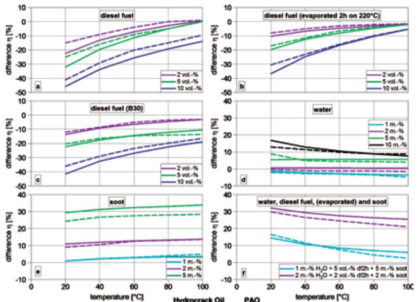
Figure 2: Influence of contamination on viscosity behavior for two base oil formulations
