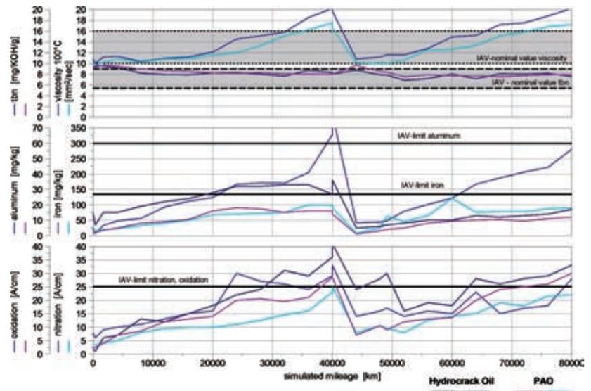
Figure 4: Influence on lubricant parameters in engine testing during a driving profile simulated on the engine test bench
