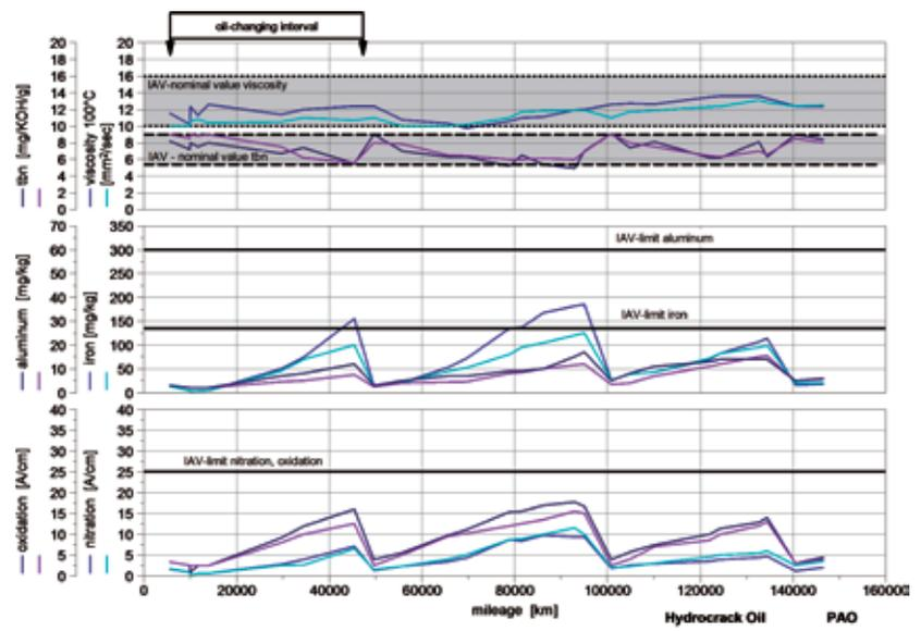
Figure 5: Influencing lubricant parameters in vehicle testing
