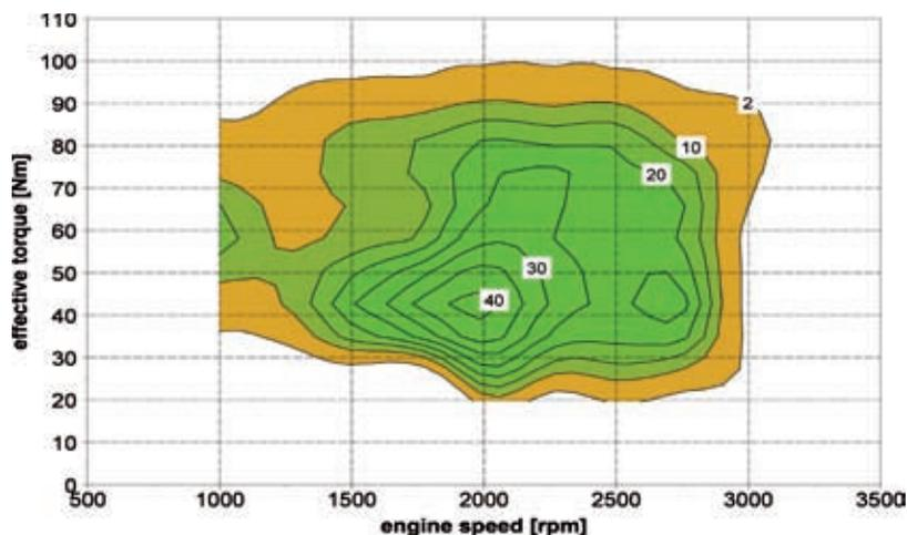
**Figure 8:** Fuel consumption advantage [g/kWh] of the early-homogeneous operating mode compared to the conventional operating mode
