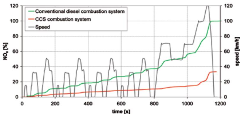
**Figure 9:** NEDC result for the CCS prototype
