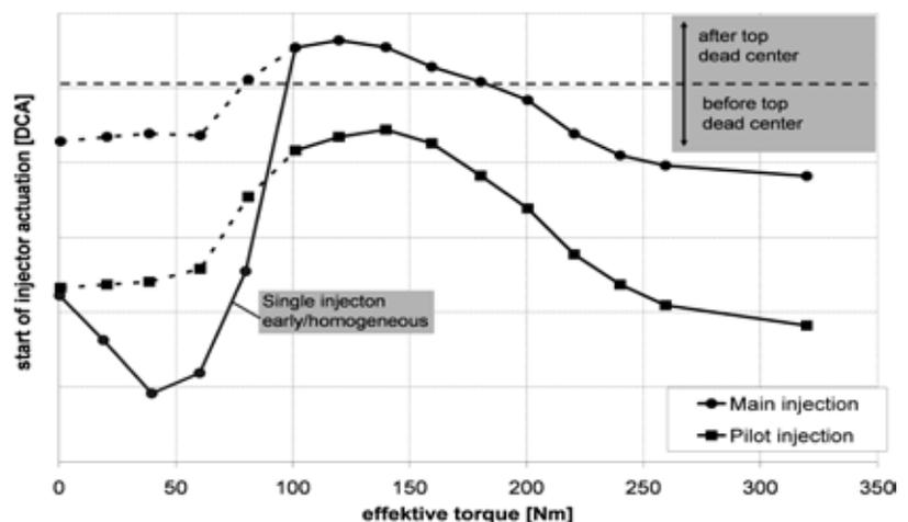
Figure 7: Injection strategy shown over an engine load cross section
