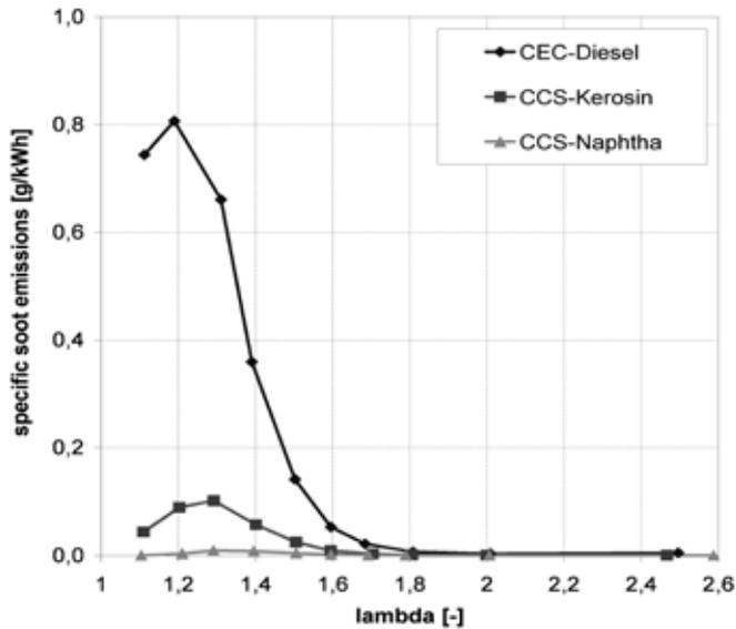
**Figure 3:** Partially homogeneous point PM – NO<sub>x</sub> trade-off (engine speed 2000 rpm; injection quantity 16.9 mg/stroke; p<sub>mi</sub> 6.9 bar)
