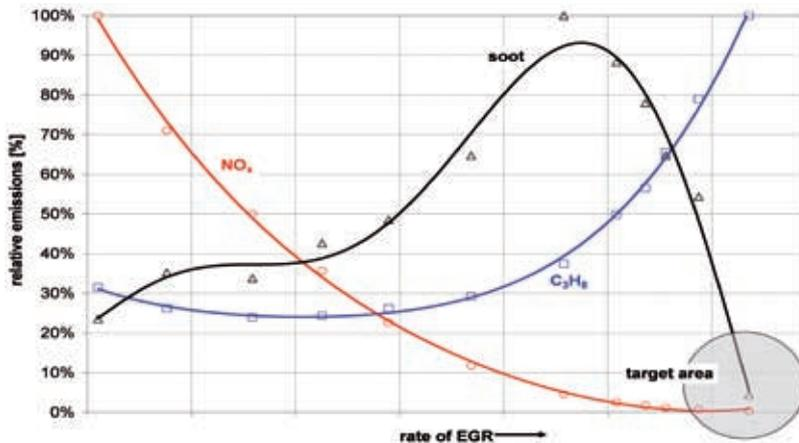
**Figure 2:** Effects of homogenisation on the formation of pollutants in diesel engine combustion (engine speed 1600 rpm; injection quantity 12 mg/stroke; p<sub>mi</sub> 3.3 bar)
