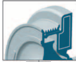
③ Adapted torsional vibration damper
