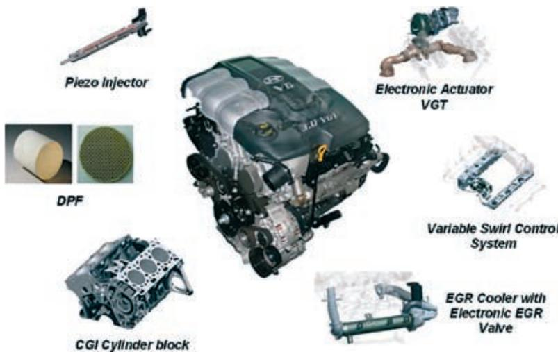
Figure 1: Main technical features of V6 3 l CRDi engine
