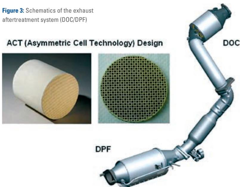
sufficient potential for Euro 4 emission standard using a diesel oxidation catalyst (DOC) only, a diesel particulate filter is provided as an optional package and further reduction of particulate matter (PM) below 5 mg/km is possible.
