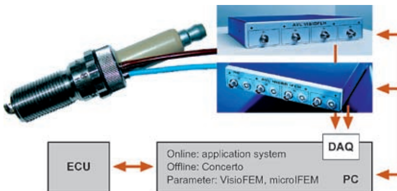
Figure 7: Configuration of on-board application system
