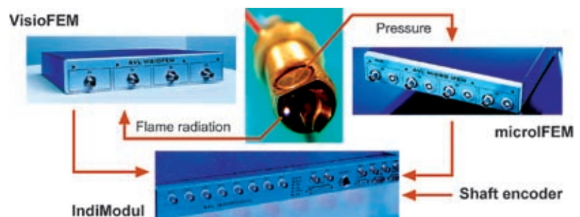
Figure 3: Pressure and flame measurement system modules
